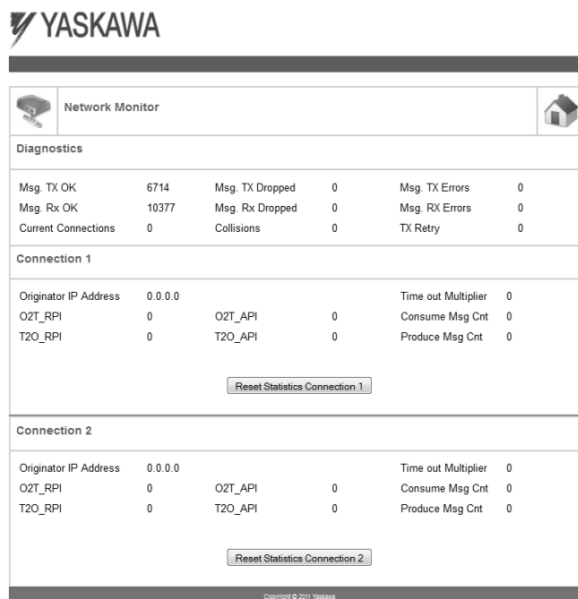
Figure 23 Network Monitor Page View
