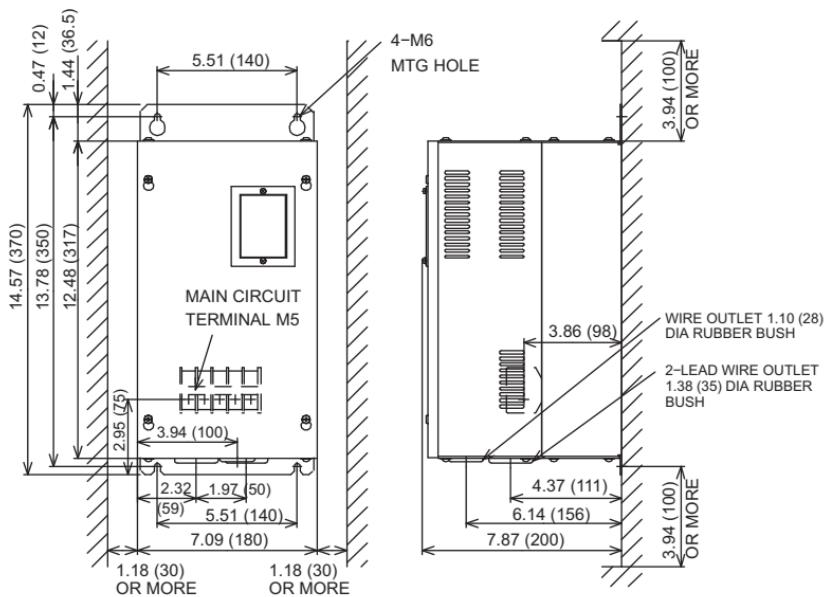
Fig. 3 Braking Unit Dimensions in inches (mm) CDBR-2045B
