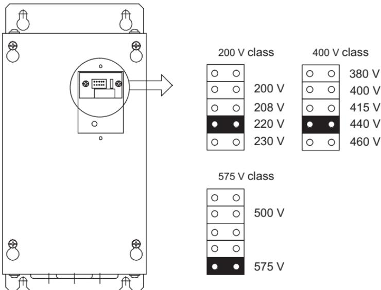
Fig. 22 Braking Unit Power Supply Voltage Selection
