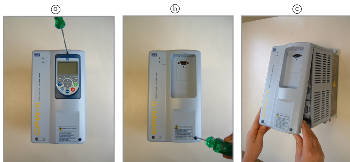
Figure 2: Removal of front cover
