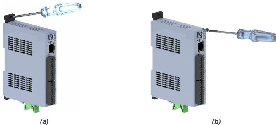
Figure 3.2: Mounting directly to the panel
