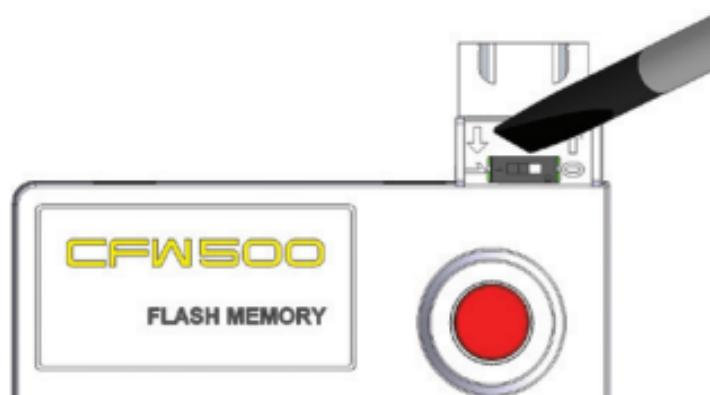
(c) Position 0: data transfer from CFW500-MMF to the CFW500
