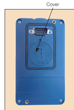
Figure 31: Keypad battery cover to access battery
