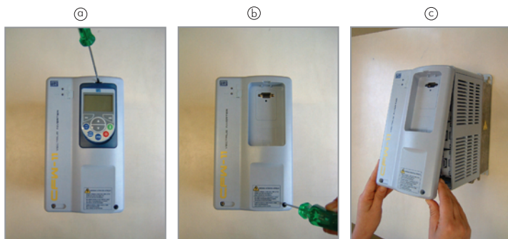
Figure 2: Removal of front cover
