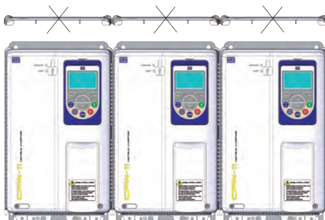
(c) Only frame sizes B and C: side-by-side mounting - No clearance required between inverters if top cover is removed
