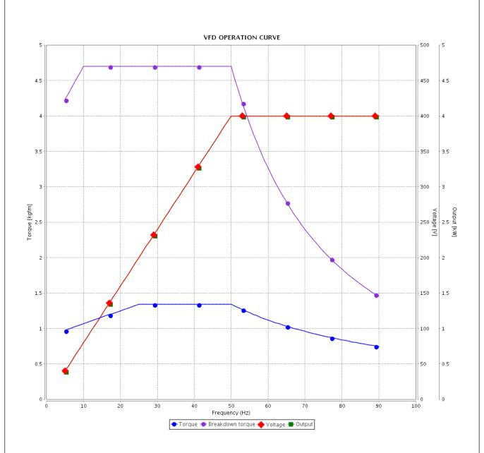
Performance : 400/690 V 50 Hz 2P : 7.59/4.40 A : 0.0081 kgm<sup>2</sup> Rated current Moment of inertia (J) **LRC** : 7.7 Duty cycle : S1 : 1.34 kgfm Insulation class : F Rated torque : 250 % Locked rotor torque Service factor : 1.00 Breakdown torque : 350 % Temperature rise : 80 K Rated speed : 2900 rpm Design
