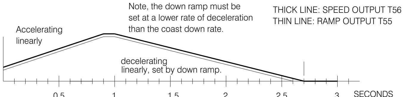
To ramp down under control of the DOWN RAMP preset, open circuit the speed reference to the drive.
