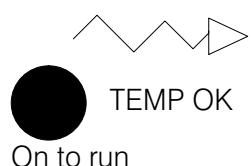
This alarm will trigger if the controllers heatsink reaches an excessive temperature. The main contactor will de-energise and the lamp will extinguish. When the heatsink has cooled down to a safe temperature the lamp will come on again. The main contactor will then be able to be energised by an external command. If this alarm is triggered then steps should be taken to improve the ventilation of the unit.
