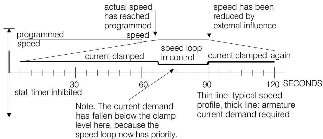
NOTES. The torque input signal is used to clamp the upper limit of the internal current demand signal before it is fed to the MAX. CURRENT presets. If the speed loop does not require current greater than the clamp level, then it will have control.
