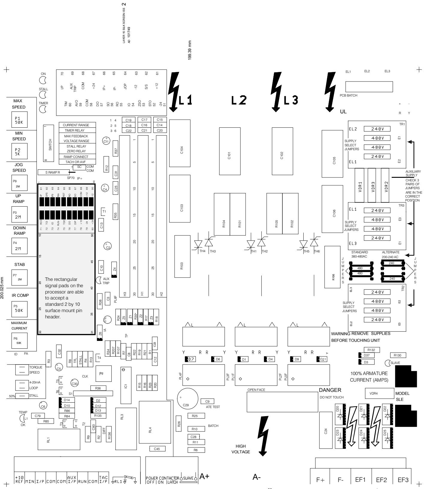
The rectangular signal pads on the processor are able to accept a standard 2 by 10 surface mount pin header.
