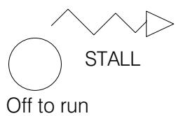
The STALL alarm is triggered by a timer according to the current demand. (150% for 30secs, 125% for 60secs, 110% for 120secs). The timer starts timing when the current demand exceeds 105%. This is indicated by the TIMER LAMP.
