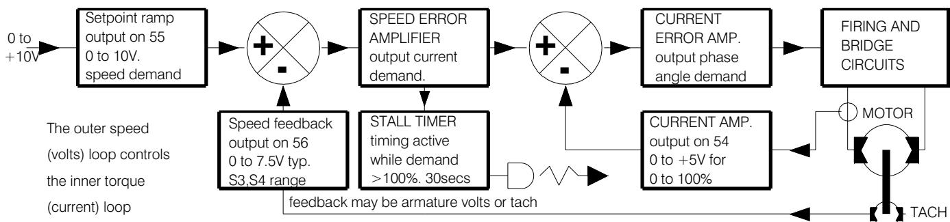
There is a comprehensive range of extra inputs and outputs and the unit has electrically isolated control circuits to allow interfacing to external sources. The units are assembled using the latest automation, and employ modern surface mount techniques. This gives superb accuracy and stability and is only made possible by the high production volumes of **SPRINT/Electric**
