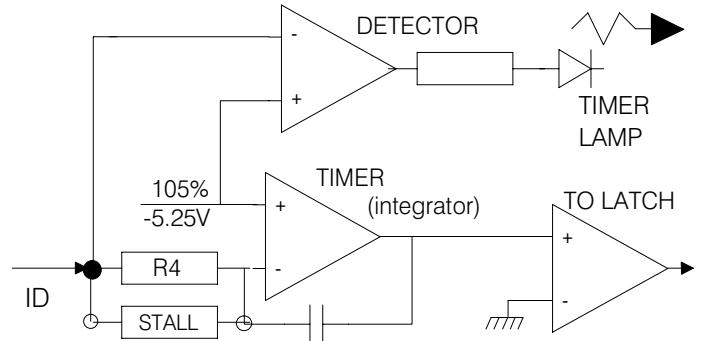
To reduce the stall time add a resistor in the stall position. See layout on page 22. 3M9 = 15secs, 2M2 = 7secs, 1M = 3secs.
