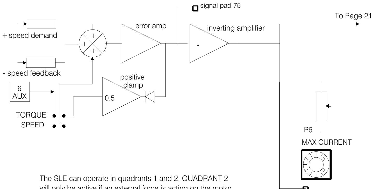
The SLE can operate in quadrants 1 and 2. QUADRANT 2 will only be active if an external force is acting on the motor to cause it to rotate in reverse.
