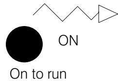
The ON lamp indicates that the auxiliary supply is energised. **WARNING:** Do not assume that the supply is disconnected if the lamp is off.
