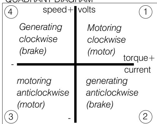
The TORQUE clamp operates in 1 and 2 on the positive current
