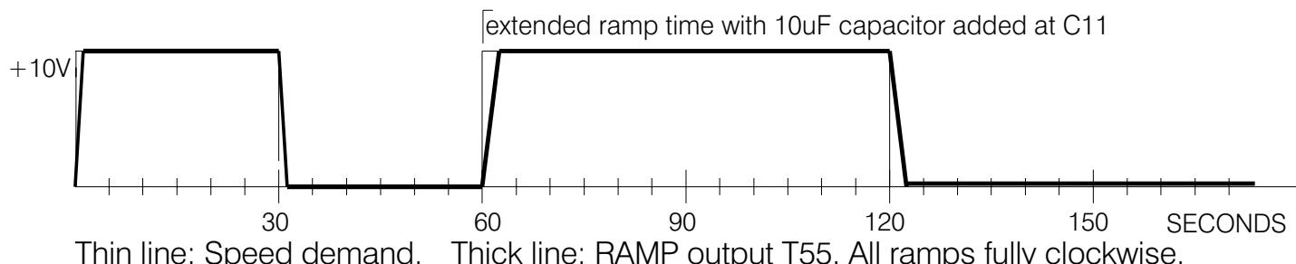
Thin line: Speed demand. Thick line: RAMP output T55. All ramps fully clockwise.
