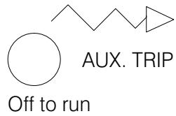
This alarm is provided for external use and is connected via terminal 69. The terminal possesses a 3K3 Ohm pull up resistor to +24V. The alarm will trigger when the resistance to 0V (com). exceeds approximately 2KOhm or the voltage on T69 exceeds 9V. The AUX TRIP input may also be used for main contactor interlock or enable relay logic.
