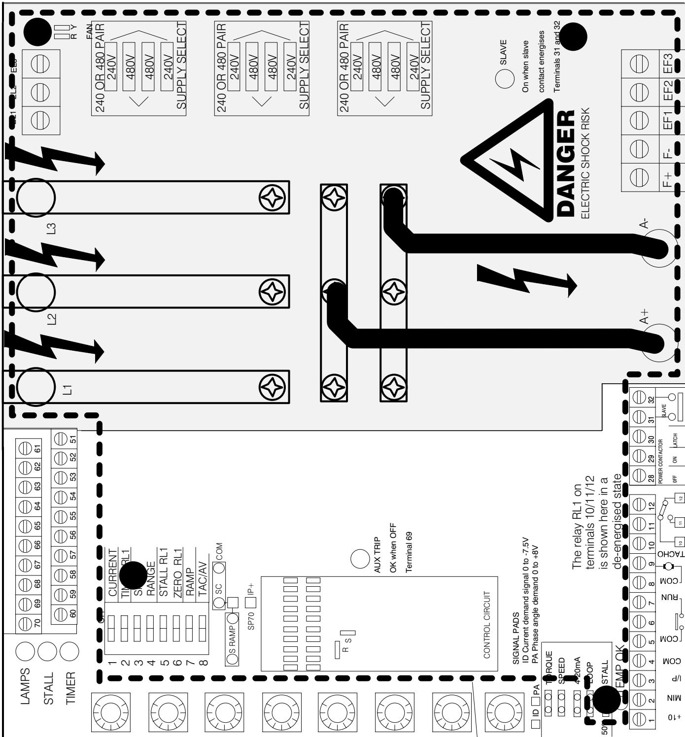
SAFETY WARNING THE SHADED AREA OF THE UNIT IS AT DANGEROUS POTENTIAL. DO NOT TOUCH ANY PART OF THE ELECTRONICS AND PRINTED CIRCUIT BOARD IN THE SHADED AREA. TAKE CARE TO KEEP CLEAR OF THE HIGH POTENTIAL AREA
