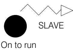
The SLAVE lamp indicates that the slave relay for the main contactor is energised, and the internal contact across terminals 31 and 32 is closed.
