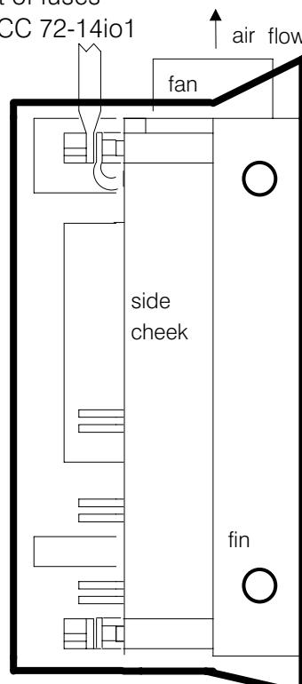
All models have auxiliary signal terminals, marked 51 to 70, on the upper edge of the card. NOTE the signal terminal numbering system is common to other SPRINT ELECTRIC drive units. Control terminal torque T51 - T70 7 lb - in. or 0.8 N - m
