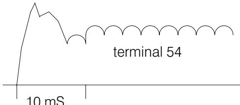
Overshoot of the current may be reduced by anticlockwise rotation of the speed stability preset.
