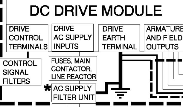
The internal earth cable must be earthed at each end. The incoming earth must be effective at RF.
