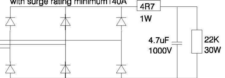
When the drive is being supplied from a local transformer, the commutation process in the thyristor bridge will cause high voltage overshoots to occur on the incoming supply. This is due to the inductance of the transformer and the lack of any other substantial load to absorb the high energy spikes.
