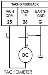
Figure 4-11: DC tachometer
