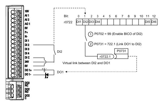
BICO or the binary interconnection technology can help the user to connect internal function and values to realize more customized features.
