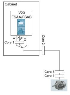
For 230 V filtered and unfiltered frame size AC inverters with the maximum motor cable length of 10  $\,\mathrm{m}$ :
