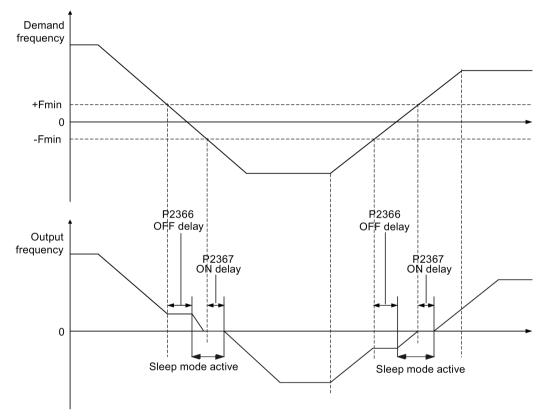
PID sleep mode (hibernation): When the inverter under PID control drops below the PID hibernation setpoint (P2390), the PID hibernation timer (P2391) is started. When the timer expires, the inverter is ramped down to stop and enters sleep mode. The inverter restarts when it reaches the PID hibernation restart point (P2392).
