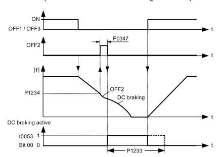
The inverter pulses are inhibited after the braking time has expired.
