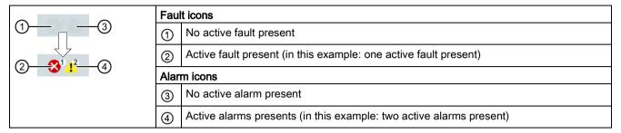
If the fault/alarm icon indicates presence of active faults/alarms, always go to the diagnostics page to view the detailed information.
