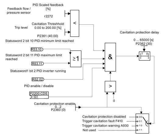
**Cavitation Protection Logic Diagram**
