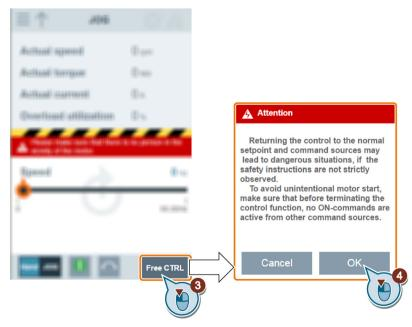
Note that before returning the control, make sure there is no inverter output and the motor stops running.
