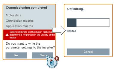
8. Confirm completion of the quick commissioning when the following window appears. If the Web page indicates that the optimization fails, you can select to try optimization again.
