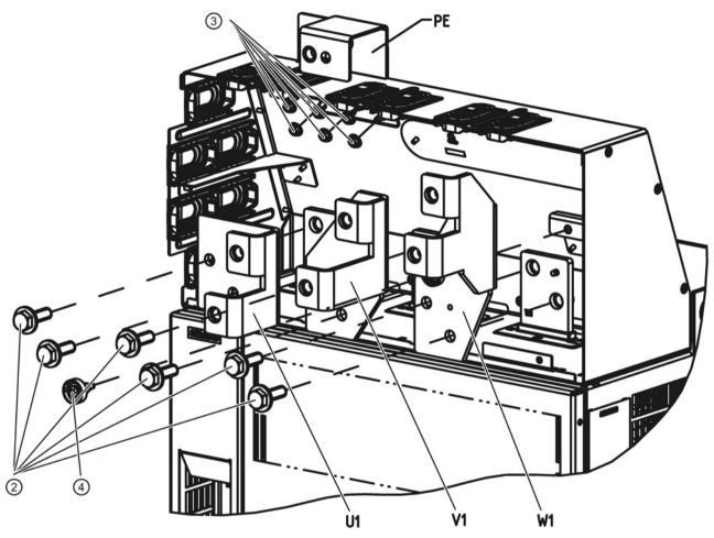
Figure 4-10 Installing the mounting kit, step 2
