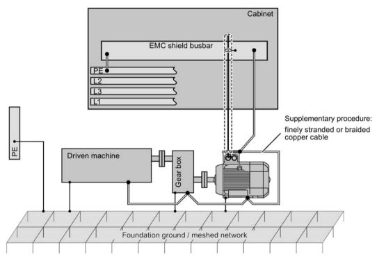
Figure 4-16 Additional high-frequency bonding of the drive system
