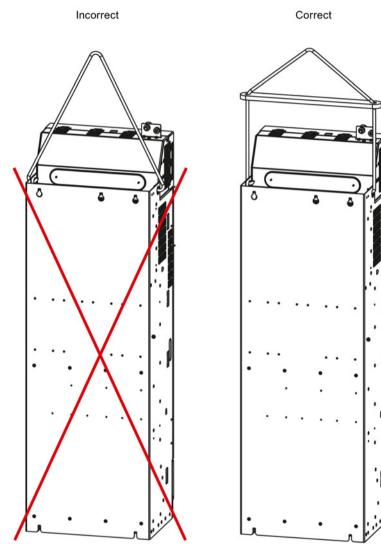
Figure 3-3 Lifting Power Modules
