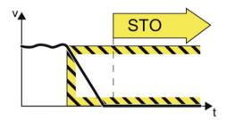
Figure 8-3 Safe Stop 1 (SS1-t, time controlled)
