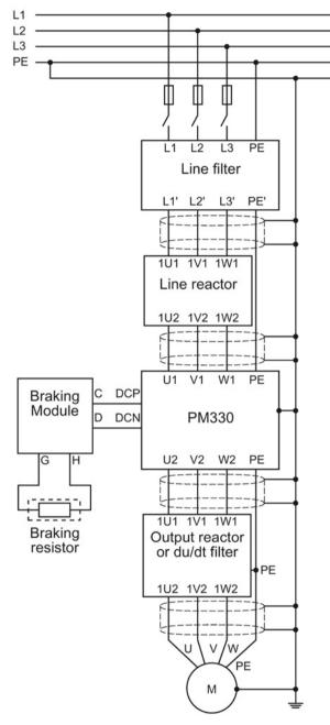
Figure 2-1 PM330 block diagram
