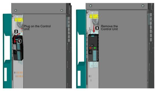
Figure 3-7 Mounting and removing the Control Unit
