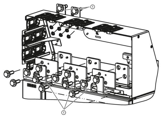
Figure 4-9 Installing the mounting kit, step 1
