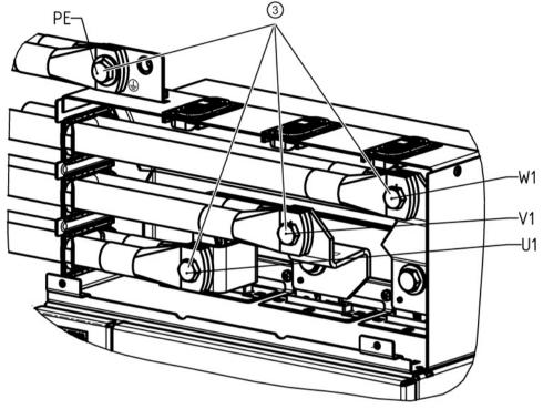
3. Final state with mounted installation set, tightening torque for the fixing screws ③: 50 Nm
