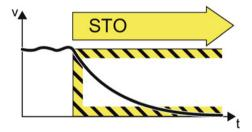
Figure 8-1 Safe Torque Off (STO)
