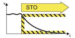
Figure 7-1 Safe Torque Off (STO)
