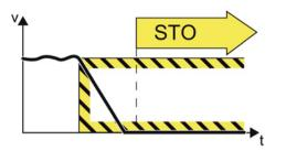
Figure 7-2 Safe Stop 1 (SS1-t, time controlled)
