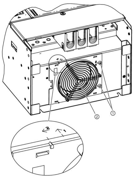
Figure 5-3 Fan removal for frame size GX, view from below
