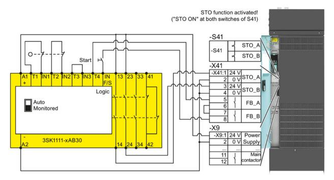
Figure A-2 3SK1 power supply via X9 from the PM330
