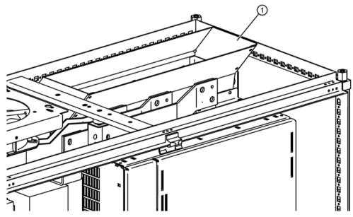
Figure 3-1 Example of an air discharge duct
