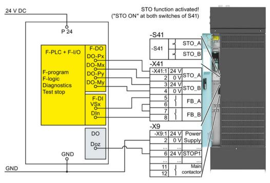
Figure A-5 SS1-t with an F-PLC
