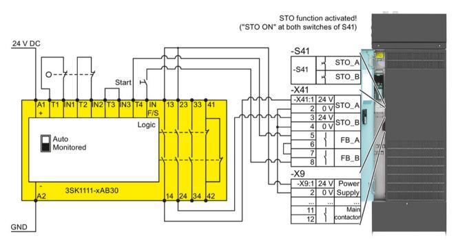
Figure 4-13 PM330 with safety relay, sensor and start button
