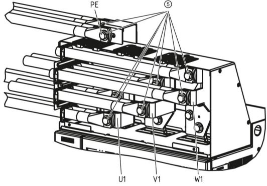
3. Final state with mounted installation set, tightening torque for the fixing screws (5): 50 Nm
