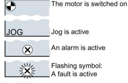
Figure 4-2 Other keys and symbols of the BOP-2 Procedure for switching the motor on and off via the operator panel:
