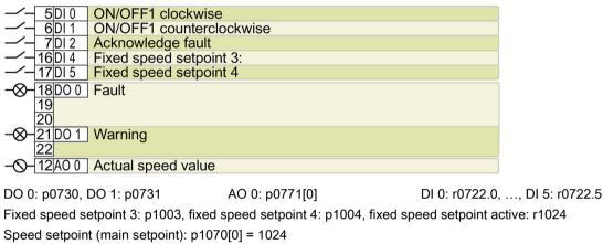
DI 4 and DI 5 = high: the inverter adds the two fixed speed setpoints
