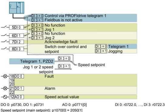
Jog 1 speed setpoint: p1058, factory setting: 150 rpm Jog 2 speed setpoint: p1059, factory setting: -150 rpm Designation in the BOP-2: FB cdS
