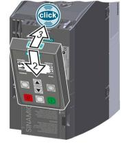
You have plugged the BOP-2 onto the inverter
