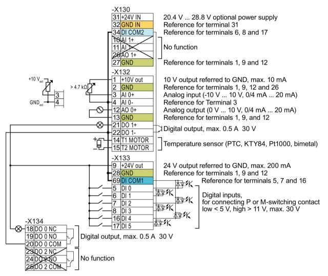
Figure 3-6 Wiring example of the digital inputs with the internal inverter 24 V power supply
