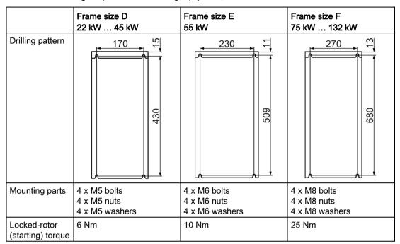
Table 3-2 Drilling templates and mounting equipment, FSD ... FSF
