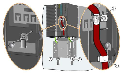
Fix the line connecting cable using a cable tie as shown in 1.
