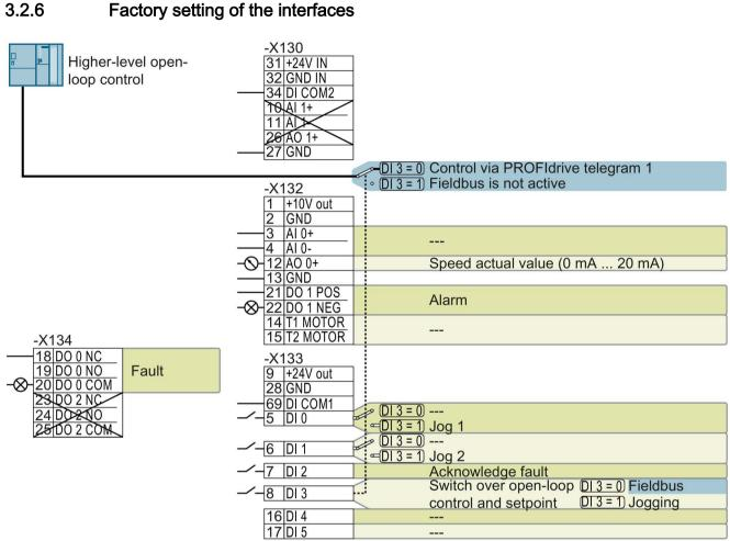
Figure 3-7 Factory setting for G120C PN, FSD ... FSF
