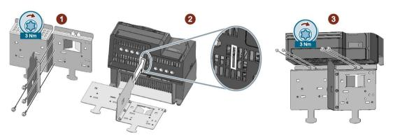
Figure 3-2 Mounting the lower shield plate, FSD and FSE
