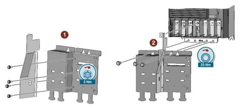
Figure 3-3 Mounting the lower shield plate, FSF
