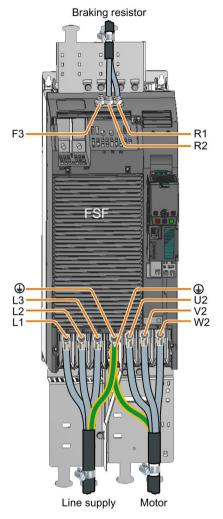
Figure 3-4 Connections for the line supply, motor and braking resistor
