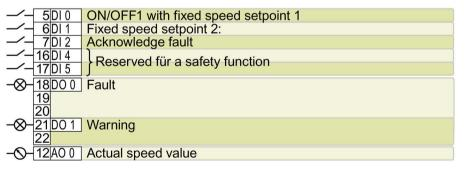
DO 0: p0730, DO 1: p0731 AO 0: p0771[0] DI 0: r0722.0, ..., DI 5: r0722.5 Fixed speed setpoint 1: p1001, fixed speed setpoint 2: p1002, fixed speed setpoint active: r1024 Speed setpoint (main setpoint): p1070[0] = 1024
