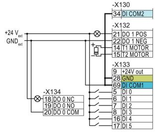
If you want to connect the potential of the external power source to the potential of the inverter's internal power supply, you must connect "GND" to terminals 34 and 69.
