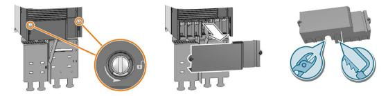
Figure 3-5 Connecting the line supply and motor, FSF
