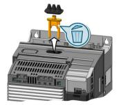
4. Adapt the seal to the cable cross-section.
