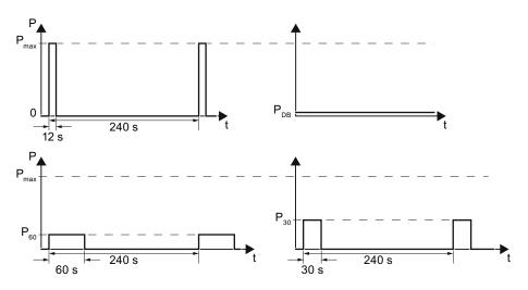
Figure 13-4 Pulse power, rated power and duty cycle examples of the braking resistor
