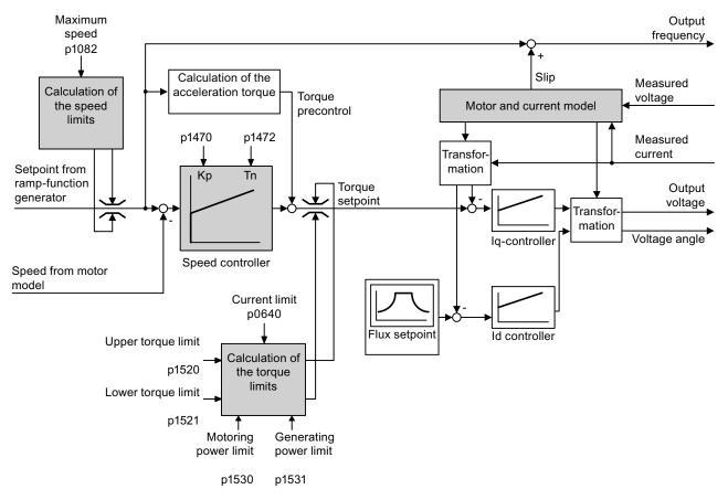
Figure 9-20 Simplified function diagram of sensorless vector control
