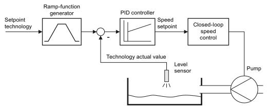
Figure 9-31 Example: technology controller as a level controller
