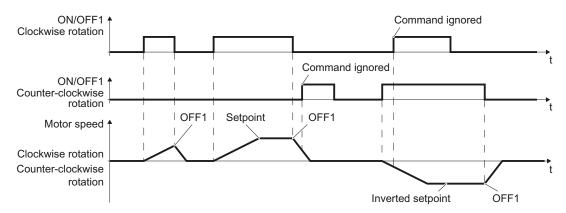
Figure 9-4 Two-wire control, method 2
