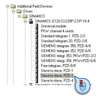
With a double-click, open the dialog box to make additional settings for the slave-to-slave communication.
