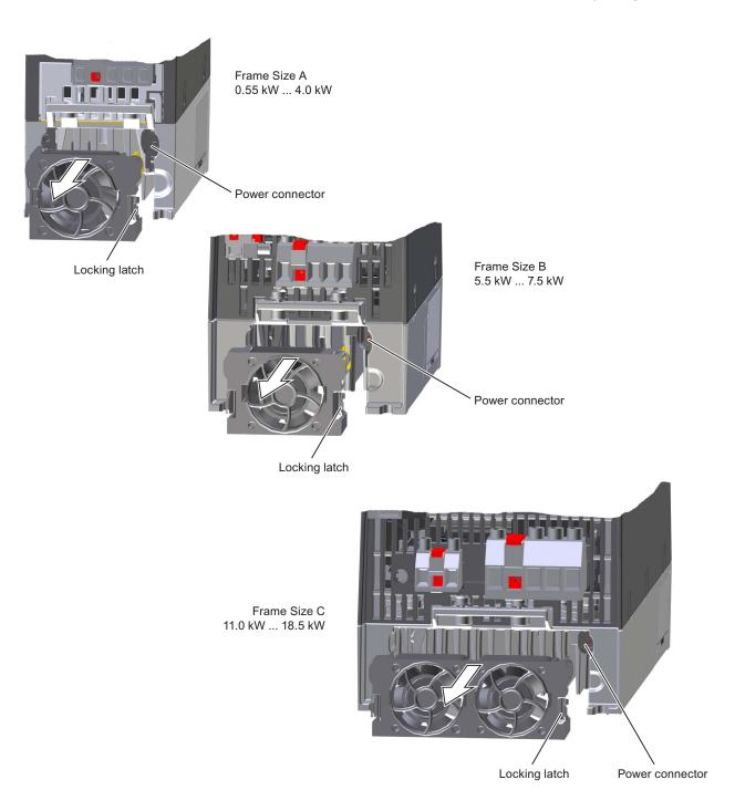
Figure 11-1 Heat sink fan replacement
