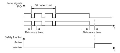
Figure 9-35 Filter for suppressing temporary signal changes
