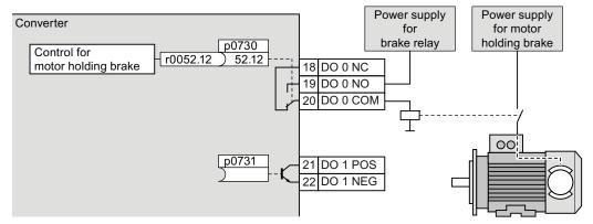
Figure 9-26 Simplified diagram of motor holding brake connected to DO 0 of the converter
