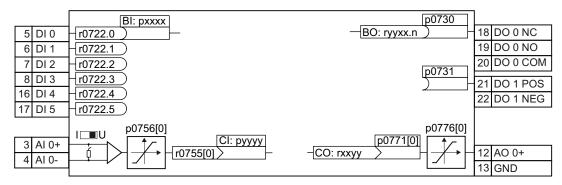
Figure 7-1 Internal connection of the inputs and outputs
