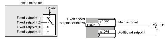
Figure 9-15 Fixed speeds as setpoint source
