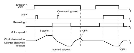
Figure 9-7 Three-wire control, method 2
