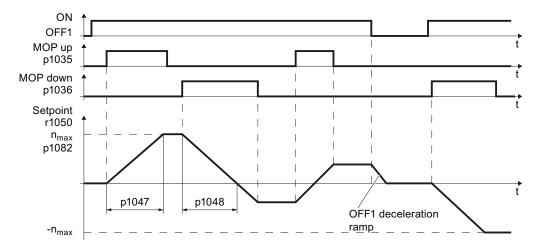
Figure 9-14 Function chart of motorized potentiometer
