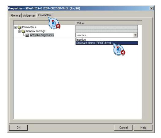
With the next ramp-up of the controller, the diagnostic messages of the converter are then transferred to the controller.
