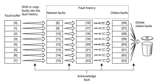
Figure 12-8 Fault history after acknowledging the faults
