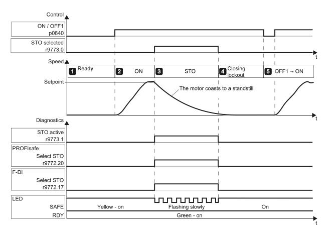
Figure 9-39 STO acceptance test for basic functions
