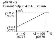
Figure 7-4 Examples for scaling characteristics
