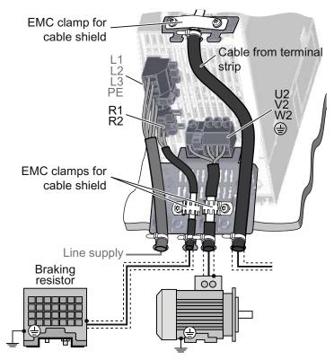
Figure 4-4 Converter shielding
