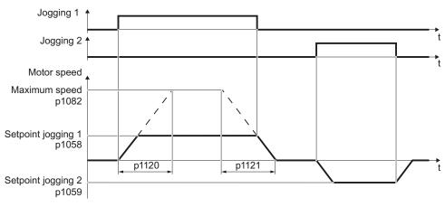
Figure 9-8 Behavior of the motor when "jogging",
