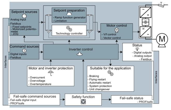
Figure 9-1 Overview of inverter functions
