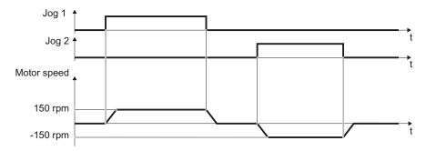
Figure 6-5 Jogging the motor in the factory setting
