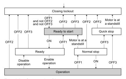
Figure 9-2 State overview of the converter
