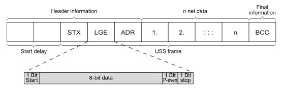
Figure 8-8 Structure of a USS telegram
