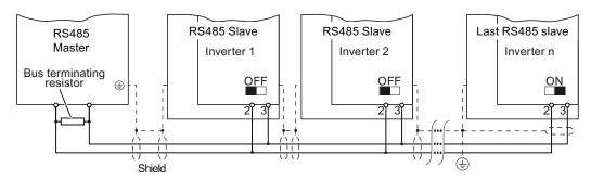
Figure 8-7 Communication network via RS485
