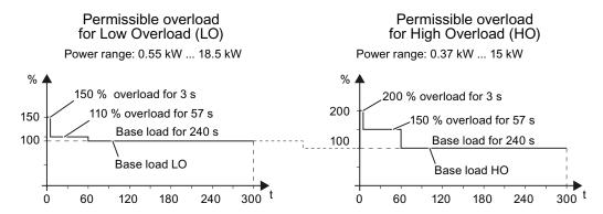
Figure 13-1 Duty cycles, "High Overload" and "Low Overload"
