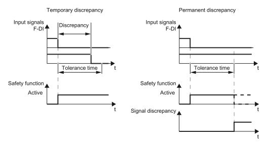
Figure 9-33 Tolerance regarding discrepancy
