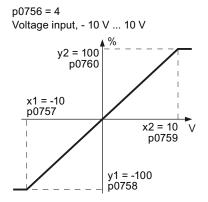
Figure 7-3 Examples for scaling characteristics
