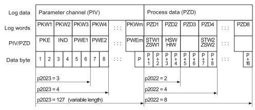
Figure 8-9 USS telegram - user data structure
