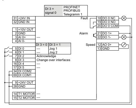
Figure 6-3 Default wiring using PROFIBUS or PROFINET communications
