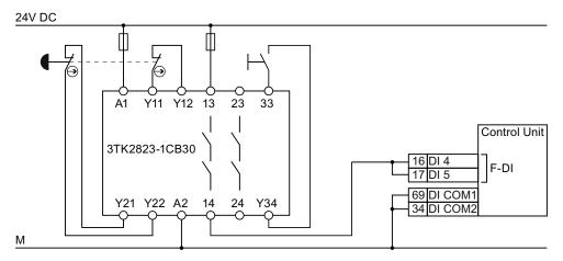
Figure A-9 Connecting a safety relay, e.g. SIRIUS 3TK28
