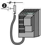
After it has been switched on, the frequency converter copies its settings to the memory card.
