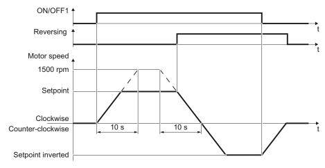
Figure 6-4 Switching on and switching off the motor and reversing in the factory setting
