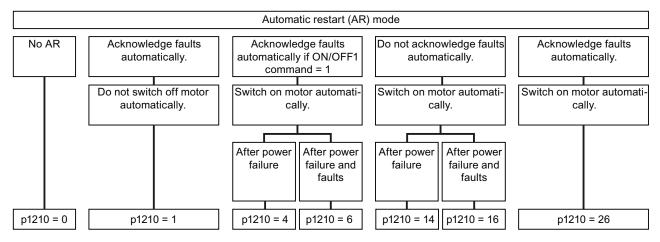
Figure 9-29 Selecting the automatic restart mode
