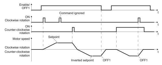
Figure 9-6 Three-wire control, method 1
