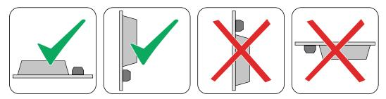
Figure 4-3 Permissible mounting orientation of the braking resistor
