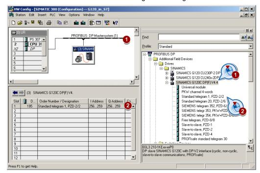
Figure A-4 Inserting a drive object
