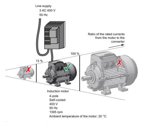
Figure 6-1 Motor data factory settings
