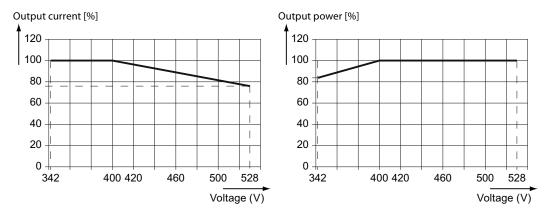
Figure 13-3 Current and Power derating required according to input voltage
