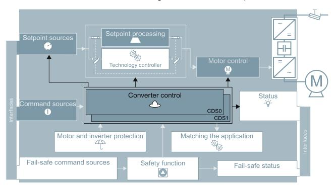
Figure 9-9 Control data set switchover in the converter
