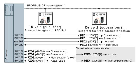
Figure A-7 Communication with the higher-level control and between the drives with slave-to-slave communication
