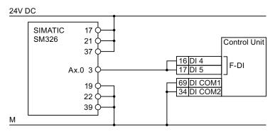
Figure A-10 Connecting an F digital output module, e.g. SIMATIC F digital output module
