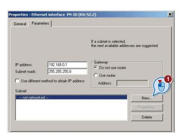
Use the "New" button (1) to either create a new PROFINET subnet or select an existing one.
