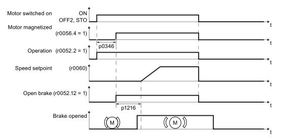
Figure 9-28 Controlling the motor holding brake after an OFF2 command or STO
