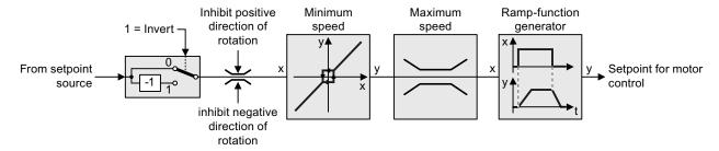
Figure 9-18 Setpoint processing in the inverter
