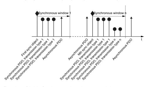
Figure 8-17 Principle of synchronous and asynchronous transmission
