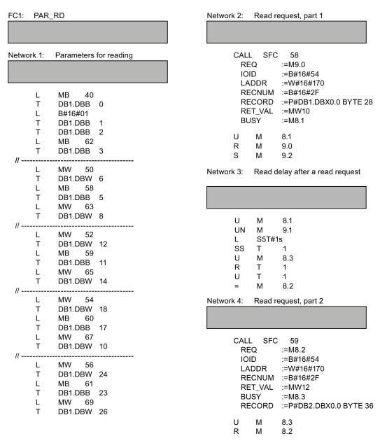
Figure A-5 Reading parameters
