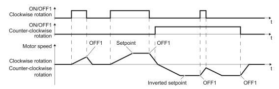
Figure 9-5 Two-wire control, method 3
