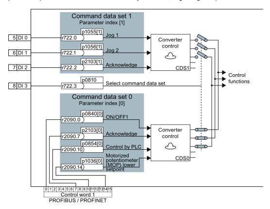
Figure 9-10 Example for the various command data sets
