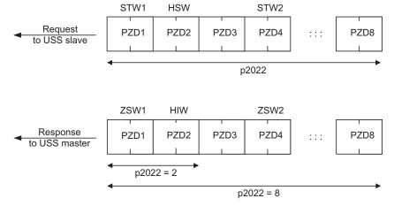
Figure 8-13 Process data channel
