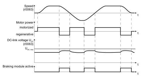
Figure 9-24 Simplified representation of dynamic braking with respect to time
