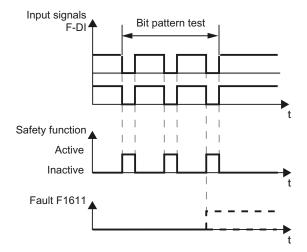
Figure 9-34 Converter response to a bit pattern test
