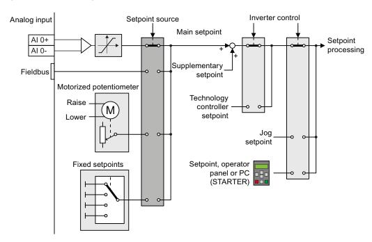
Figure 9-11 Setpoint sources for the inverter
