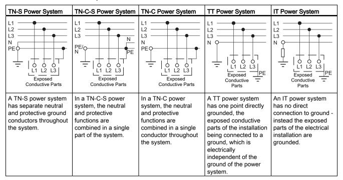
IT supplies are fully isolated from the protective earth system, usually by an isolating transformer. It should be noted, however, that a protective earth is still provided.
