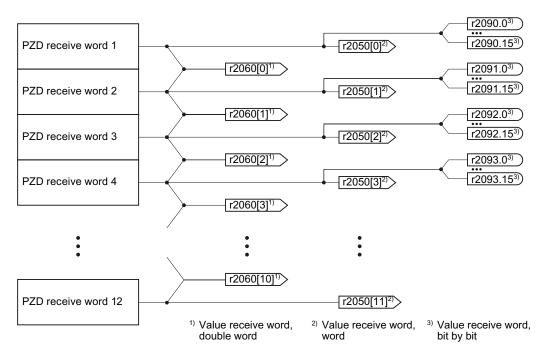
Figure 8-3 Interconnection of the receive words
