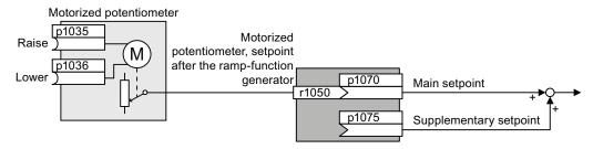
Figure 9-13 Motorized potentiometer as setpoint source
