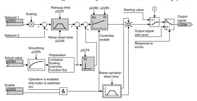
Figure 9-32 Simplified representation of the technology controller
