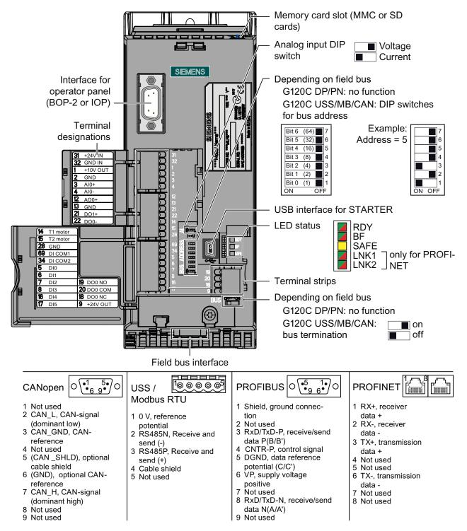
Figure 4-8 Interfaces and connectors
