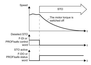
If no motor holding brake is present, the motor coasts to a standstill.
