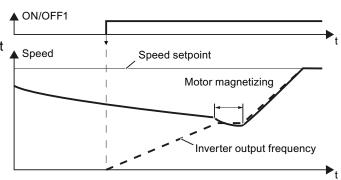
If the inverter simultaneously drives several motors, then you must only use the "flying restart" function if the speed of all of the motors is always the same (group drive with a mechanical coupling).
