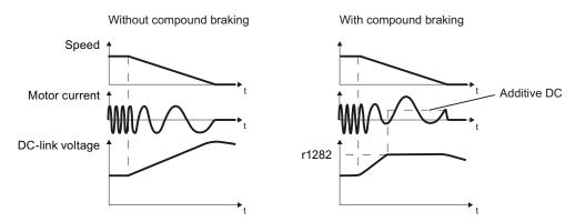
Figure 9-23 Motor brakes with and without active compound braking
