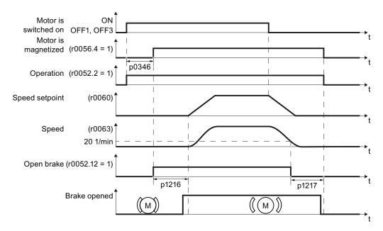
Figure 9-27 Controlling the motor holding brake when the motor is switched on and off
