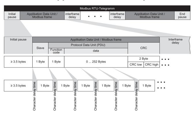
Figure 8-16 Modbus with delay times
