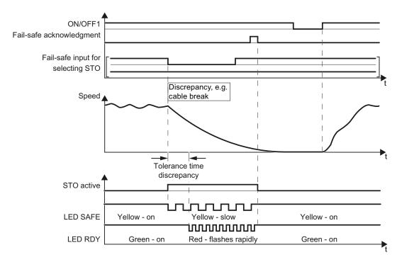
Figure 5-38 Response of safety function STO in the event of a discrepancy
