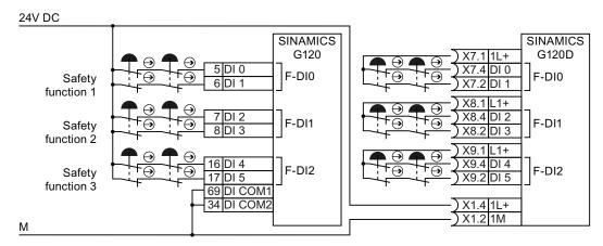
Figure 3-4 Connecting electromechanical sensors to an external power supply in series
