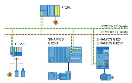
Figure 3-18 PROFIsafe communication between F-CPU and converter
