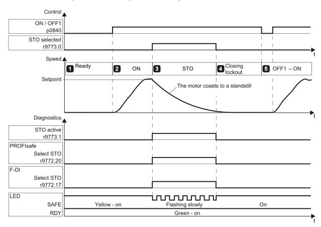
Figure 4-25 STO acceptance test for basic functions
