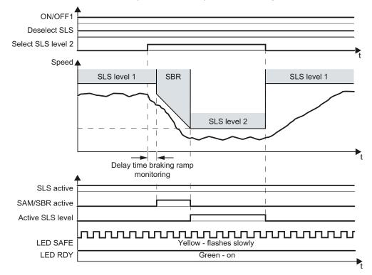
Figure 5-6 Switching between different monitoring thresholds
