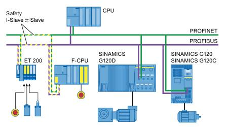
Figure 3-20 No PROFIsafe communication between F-CPU as I-slave and converter
