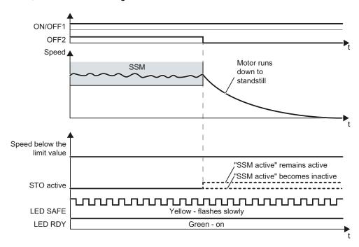
Figure 5-18 The feedback signal from SSM is "frozen" for a motor which has been switched off
