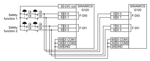
Figure 3-5 Simultaneous activation of several converters with converter power supply
