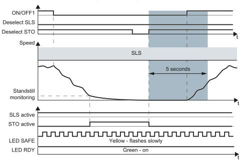
Figure 5-15 Switching the motor off and on (ON/OFF1) when SLS is active
