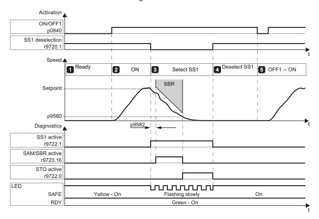
Figure 4-27 SS1 acceptance test with braking ramp monitoring
