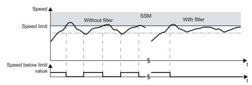
Figure 4-19 Mode of operation of the filter of the SSM function
