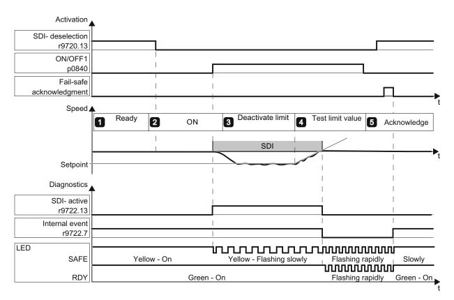
Figure 4-36 SDI acceptance for a negative direction of rotation; "SDI active" becomes inactive when the motor is switched off
