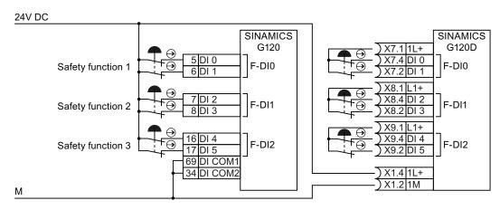
Figure 3-2 Connecting an electromechanical sensor to an external power supply
