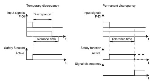
Figure 4-1 Tolerance regarding discrepancy
