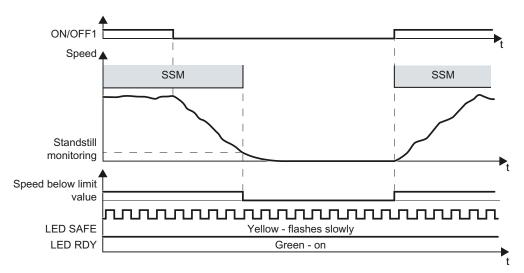
Figure 5-19 Switching the motor on and off with SSMactive, interrupting SSM
