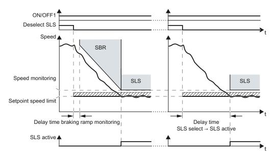
Figure 4-17 Behavior after selecting SLS. Left: with braking ramp monitoring; right: without braking ramp monitoring
