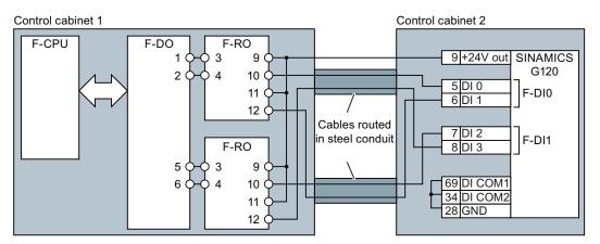
Figure 3-14 Interconnecting the converter and I/O modules in separate control cabinets
