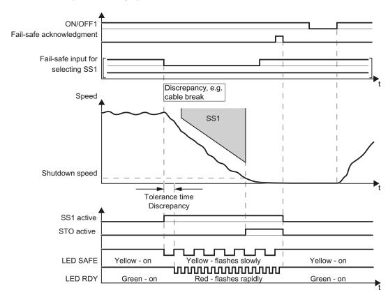
Figure 5-39 Response of safety function SS1 in the event of a discrepancy (as example: SS1 with braking ramp monitoring)
