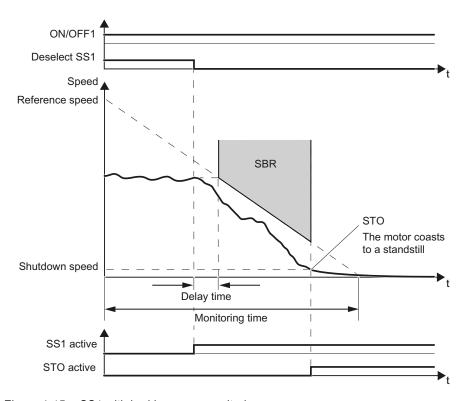
Figure 4-15 SS1 with braking ramp monitoring
