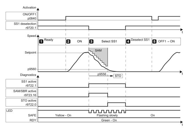
Figure 4-28 SS1 acceptance test with acceleration monitoring
