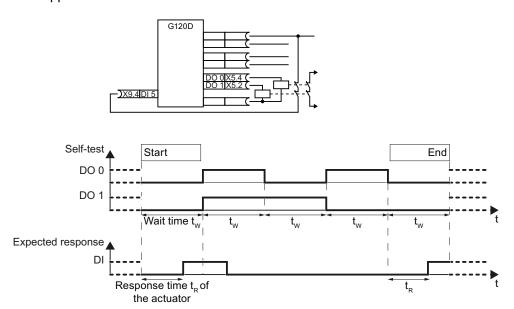
Figure 4-11 Expected response at the digital input for test mode 2
