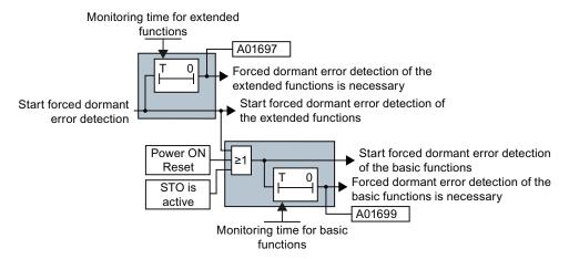
Figure 4-7 Triggering and monitoring the forced checking procedure
