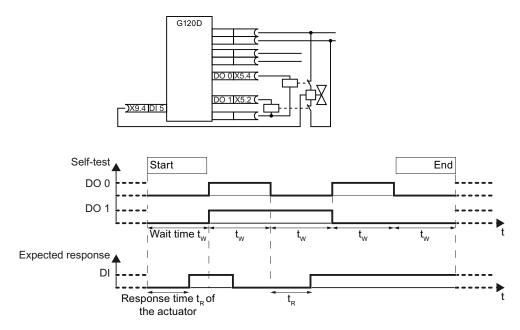
Figure 4-12 Expected response at the digital input for test mode 3
