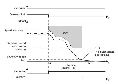
Figure 4-16 SS1 with acceleration monitoring
