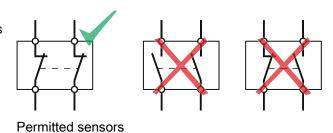
If you interconnect pre-processing safety relays via two separate cables with the converter, the two transferred must always have the same signal state.
