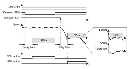
Figure 4-21 Delay time and tolerance
