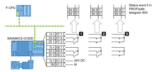
Figure 4-37 Acceptance test for the status of the fail-safe inputs using the example of aSINAMICS G120D
