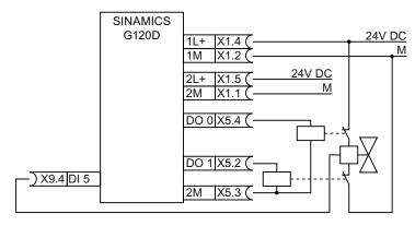
Figure 3-16 Connecting the F-DO of the G120D, mode3
