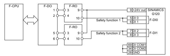
Figure 3-13 Interconnecting the converter and I/O modules within the same control cabinet
