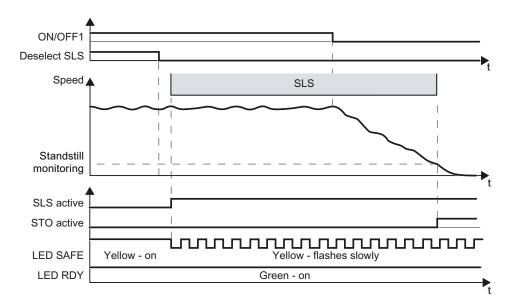
Figure 5-13 OFF1 command when the SLS safety function is active
