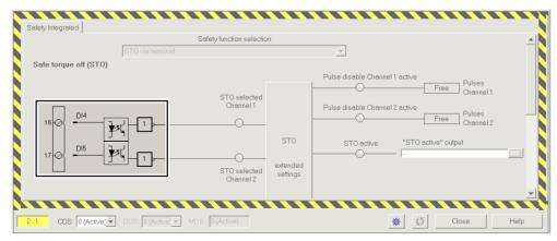
Example: automatic assignment of digital inputs DI 4 and DI 5 with STO Figure 4-23
