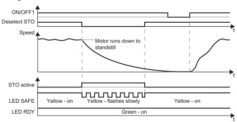
Figure 5-1 Time response of the safety function STO (Safe Torque Off)
