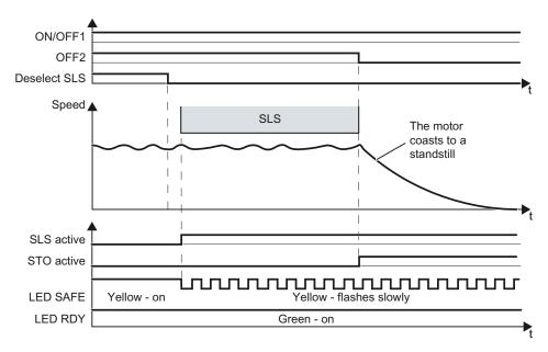
Figure 5-14 OFF2 command while the SLS safety function is active
