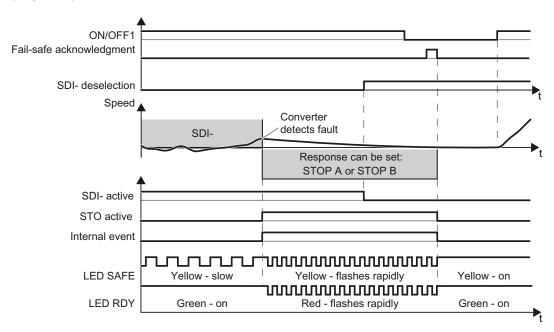
Figure 5-46 Fault response of the SDI safety function
