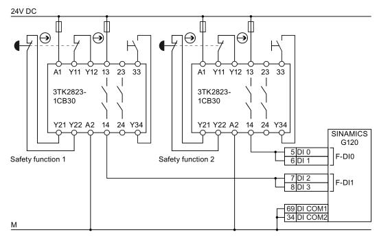
Figure 3-7 Interconnecting the converter and safety relay within the same control cabinet
