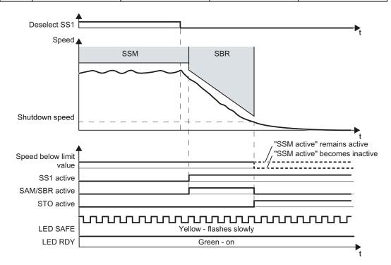
Figure 5-31 SS1 select when active SSM
