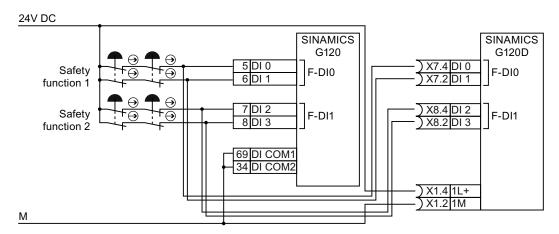
Figure 3-6 Simultaneous activation of several converters with external power supply
