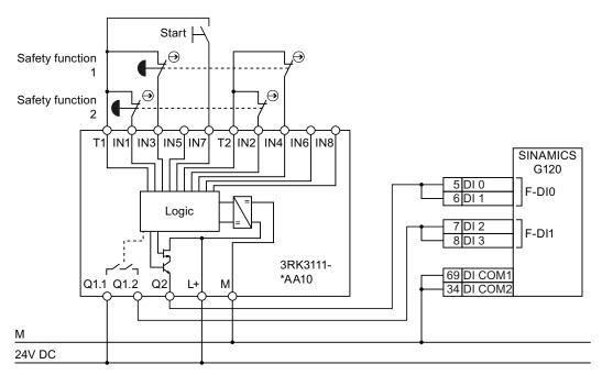
Figure 3-9 Interconnecting the converter and Modular Safety System within the same control cabinet
