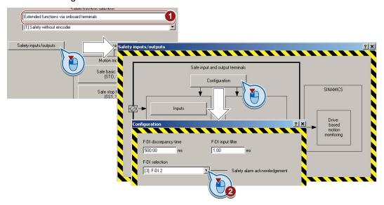
② Select a free fail-safe input for acknowledging. If there are no free fail-safe inputs available, you have to acknowledge the safety function faults using a different method. See also Section: Fail-safe acknowledgment (Page 193).
