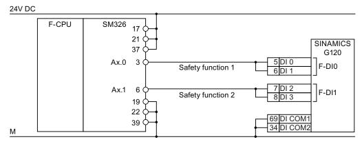
Figure 3-11 Interconnecting the converter and SM326 I/O module within the same control cabinet
