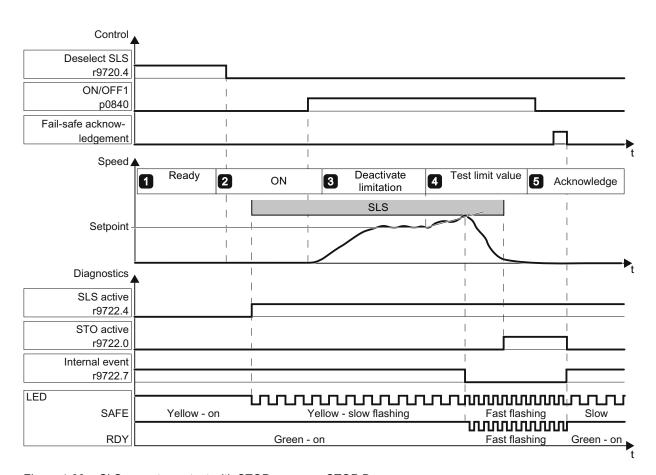
Figure 4-30 SLS acceptance test with STOP response STOP B
