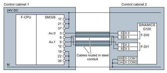
Figure 3-12 Interconnecting the converter and SM326 I/O module in separate control cabinets
