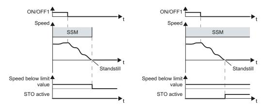
Figure 4-20 Behavior when the motor is switched off. Left: SSM is inactive. Right: SSM remains active
