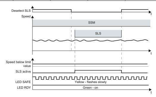
Figure 5-33 SLS select when active SSM
