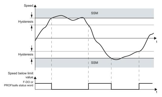
Figure 2-3 Time response of the safety function SSM (Safe Speed Monitor)
