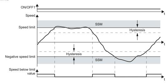
Figure 4-18 Time response of the safety function SSM (Safe Speed Monitor)
