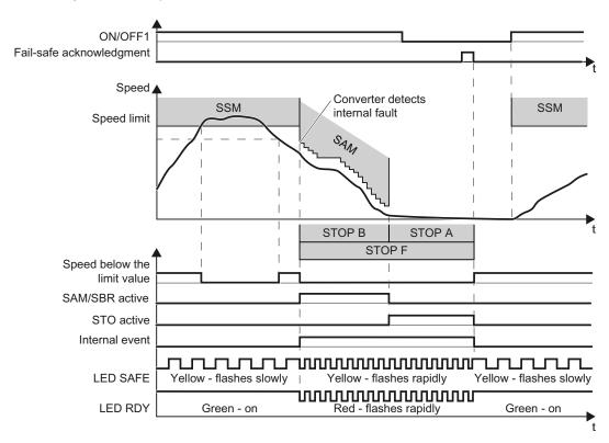
Figure 5-43 Reaction of the SSM safety function to an internal event
