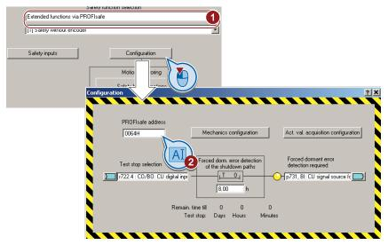
② STARTER only shows this input field if you have selected the extended functions via PROFIsafe ① (or via PROFIsafe and onboard terminals).
