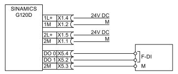
Figure 3-17 Connecting the F-DO of the G120D, mode4
