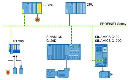
Figure 3-19 Bus configuration, shared device
