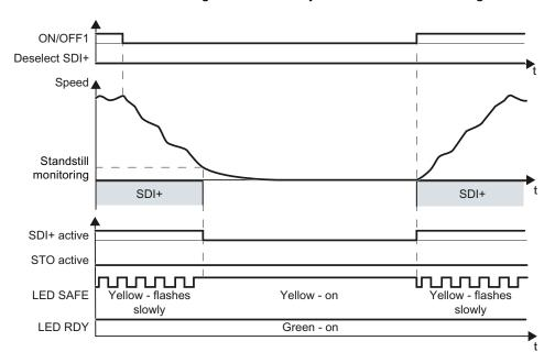
Figure 5-23 Switching the motor off and on again with SDI, active, interrupting the feedback signal from SDI
