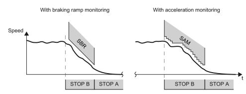
Figure 5-36 Monitoring the speed for a STOP B
