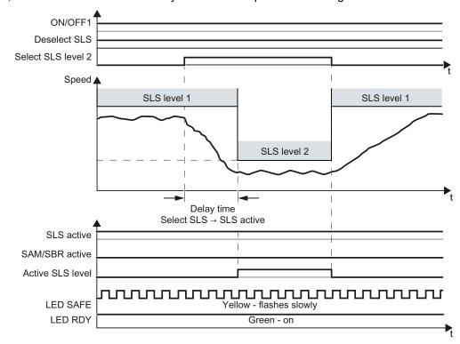
Figure 5-9 Switching between different monitoring thresholds
