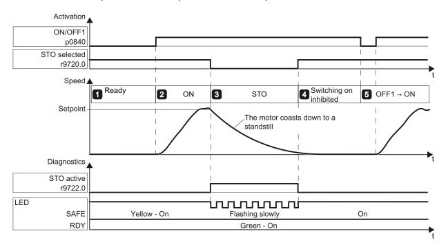
Figure 4-26 STO acceptance test for extended functions
