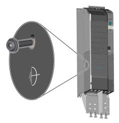
Figure 4-2 Remove screw for functional grounding
