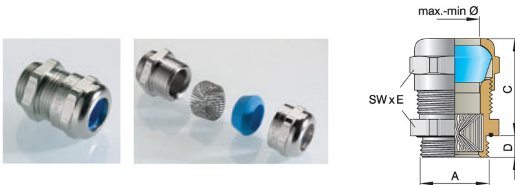
Brass-nickel plated EMC cable gland with metric thread as per EN50262. IP68 protection with up to 15 bar pressure.
