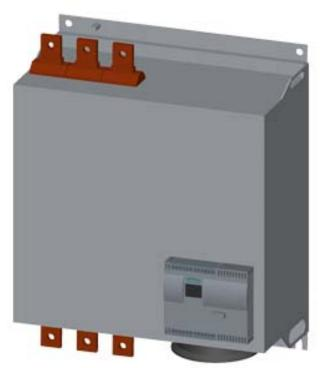
SIRIUS soft starter Values at 400 V, 40 °C Standard: 551 A, 315 kW Inside-delta: 954 A, 560 kW 200-460 V AC, 230 V AC Screw terminals
