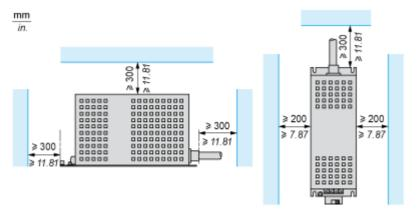
Sinus filters emit considerable heat and must not be placed underneath the drive
