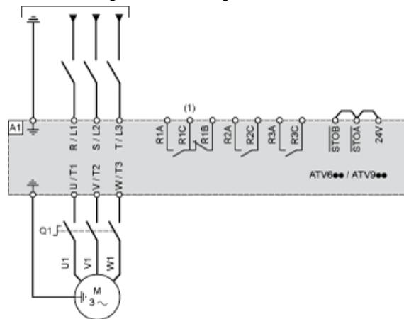
(1) Use digital output R1 set to operating state Fault to switch Off the product once an error is detected.
