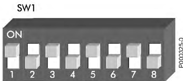
Figure 188: DIP-switch SW1 setting in three-channel mode
