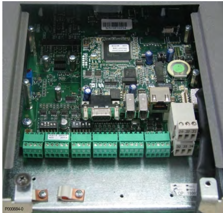
Figure 159: ES851 DataLogger fitted into slot B
