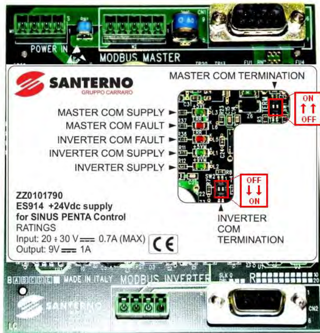
Figure 182: Position of the LEDs and DIP-switches in ES914 board
