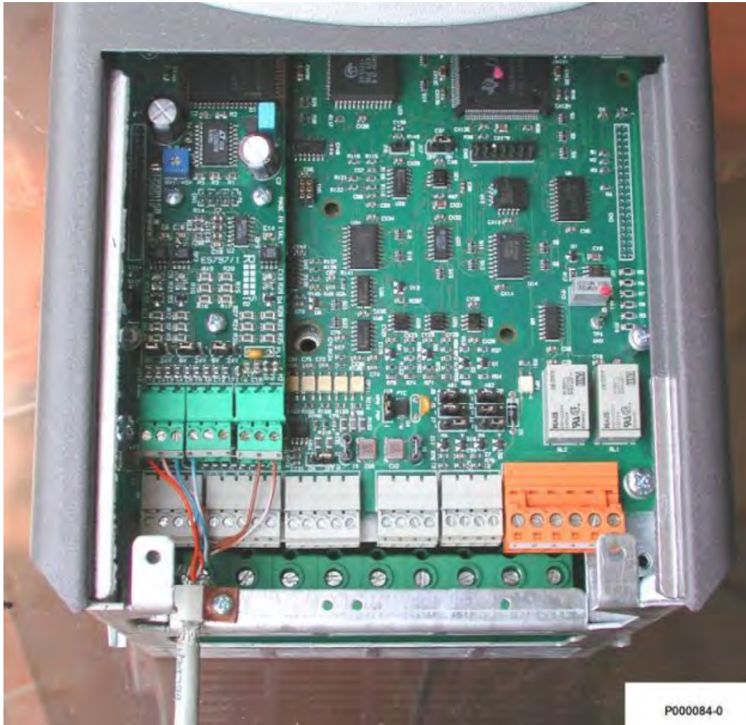
Figure 121: Wiring the encoder cable
