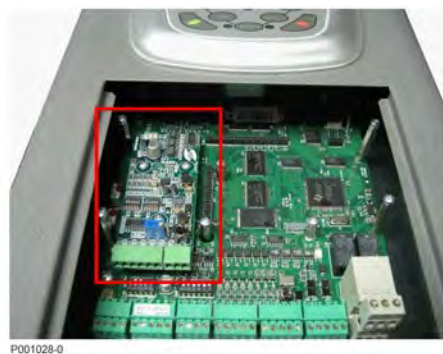
Figure 124: Encoder board fastened to its slot
