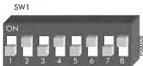
Figure 189: DIP-switch SW1 setting for five-channel mode
