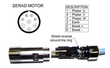
Attention. Care must be taken when making connection to connector X10. An incorrect connection can seriously damage the drive. Dangerous voltages are present on X10.
