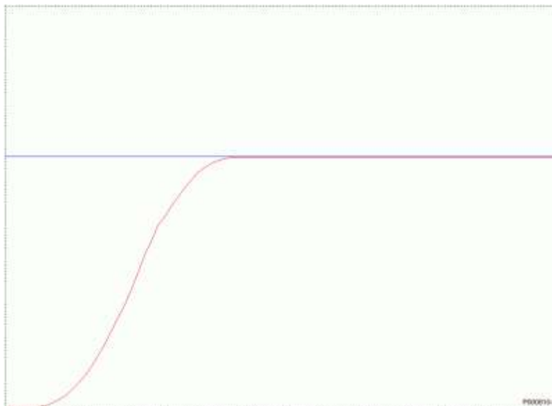
Figure 27: Response to a system tuned with the method of Ziegler and Nichols
