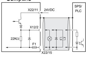
The outputs are short circuit proof; a short circuit generates an error.
