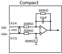
IN0 to IN3 do have the same wiring! Pin assignment X1
