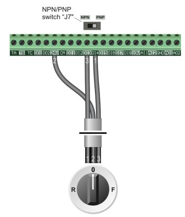
Switch, 3 Position Normally Open "Run Forward / Stop / Run Reverse"
