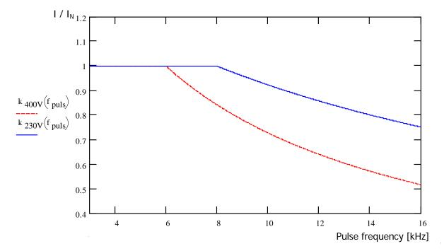
Figure 18: Heat losses due to pulse frequency
