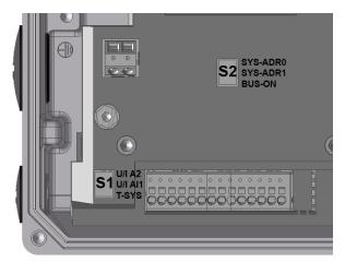
As delivered, all DIP switches are in the "0" ("OFF") position.
