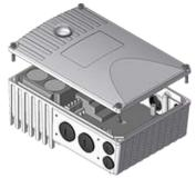
4. Fit the casing of the SK 1x0E to the terminal box base of the NORD motor using the existing screws and seal as well as the provided toothed contact washers. When doing this, align the casing so that the rounded side is facing the direction of the A bearing cover of the motor. Carry out mechanical adaptation using the "Adapter kit" ( Section 2.1.1.1 "Adapters for different motors"). With motors made by other manufacturers, it must be checked whether they can be attached.
