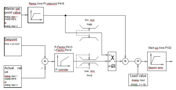
Fig.: Process controller flow-chart
