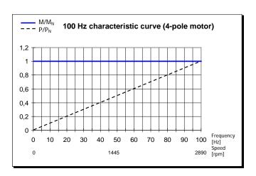
Figure 23: 100 Hz characteristic curve
