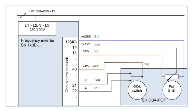
Figure 13: Wiring diagram SK CU4-POT, example SK 1x0E
