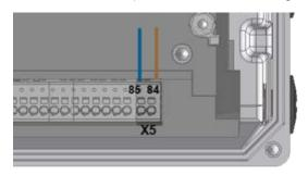
Figure 14: Connecting terminals AS-i
