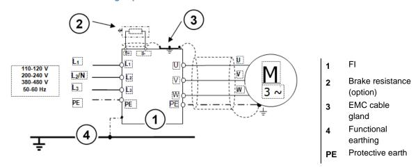
Figure 17: Wiring recommendation
