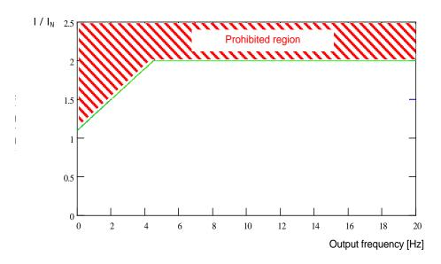
The upper limiting values for the various pulse frequencies can be obtained from the following tables. In all cases, the value (10 ... 201) which can be set in parameter P537, is limited to the value stated in the tables according to the pulse frequency. Values below the limit can be set as required.
