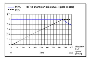
Figure 22: 87 Hz characteristic curve
