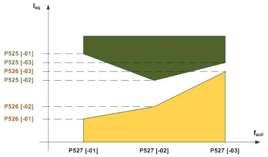
The time after which a fault is triggered can be set with parameter (P528). If the permissible range is exceeded (Example diagram: Infringement of the area marked in yellow or green), the error message E12.5 is generated unless parameter (P529) does not suppress the triggering of an error.
