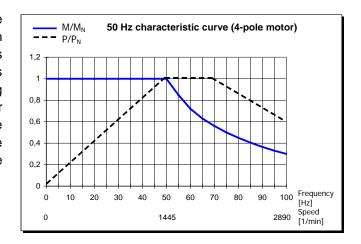
Figure 21: 50 Hz characteristic curve
