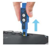
Figure 10: Disconnecting the RJ12 port
