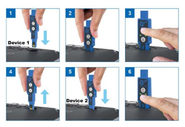
Figure 11: Data transfer procedure
