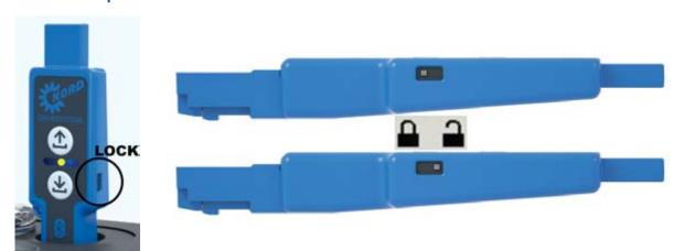
Figure 3: Write protection LOCK
