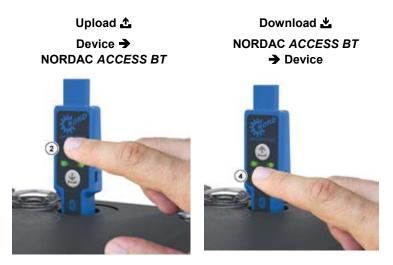
Figure 8: Data transfer, upload and download
