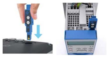
Figure 7: RJ12 connection to the device
