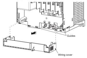
Pull out the cover along the guides in the direction shown by the arrow in the figure above.
