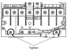
Fit the cover to the inverter along the guides.
