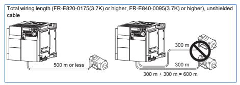
When driving a 400 V class motor by the inverter, surge voltages attributable to the wiring constants may occur at the motor terminals, deteriorating the insulation of the motor. In this case, take one of the following measure.
