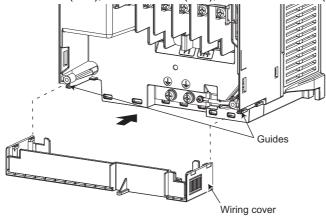
Fit the cover to the inverter along the guides.
