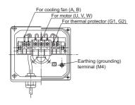
Make sure to earth (ground) the earth (ground) terminal of the flange section as well as the earth (ground) terminal in the terminal box.
