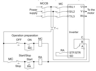
\*1 When the power supply is 400 V class, install a stepdown transformer.
