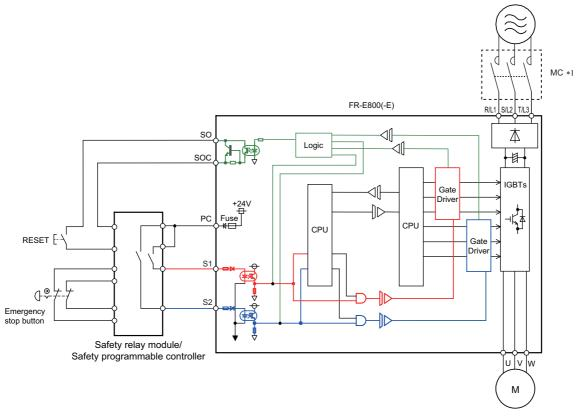
\*1 To avoid an electric shock hazard, install a magnetic contactor (MC) at the input side of the inverter.
