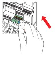
When using single wire or stranded wire without crimp terminal, push an open/close button all the way down with a flathead screw driver, and insert the wire.
