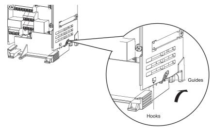
Fit the cover to the inverter along the guides in the direction shown by the arrow in the figure above.
