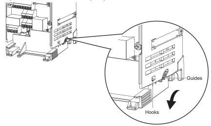
Pull out the cover along the guides in the direction shown by the arrow in the figure above.
