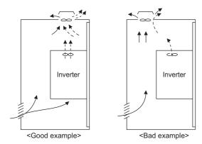
Arrangement of the ventilation fan and inverter
