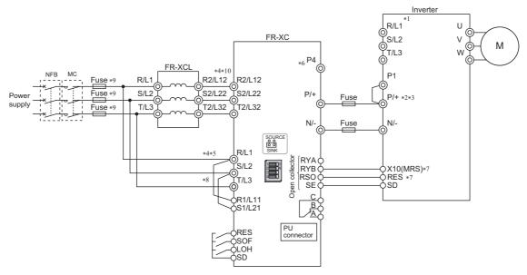
\*1 Never connect the power supply to terminals R/L1, S/L2, and T/L3 on the inverter. Doing so will damage the inverter and the converter.
