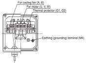
Make sure to earth (ground) the earth (ground) terminal of the flange section as well as the earth terminal in the terminal box.
