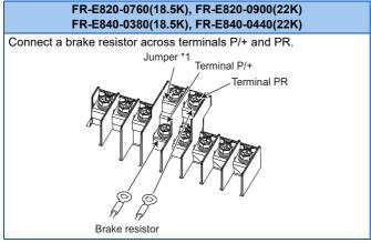
\*1 Do not remove the jumper across terminals P/+ and P1 except when connecting a DC reactor (FR-HEL).
