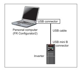
To communicate with FR Configurator2 by the USB connection between the inverter and a personal computer, use the USB mini B connector at the inverter side
