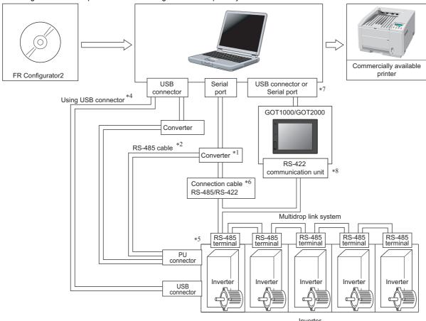
st 1 When using serial port of a personal computer, a commercially available converter is required.
