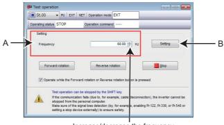
Increase/decrease the frequency (rotation speed, machine speed) in minimum increments.
