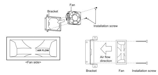
(2) Attach the bracket to the inverter.
