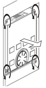
To reinstall the operation panel, align its connector on the back with the PU connector of the inverter, and insert the
