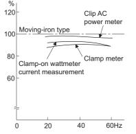
Example of measuring inverter output current
