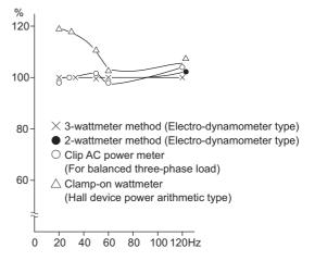
Example of measuring inverter input power
