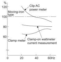
Example of measuring inverter input current
