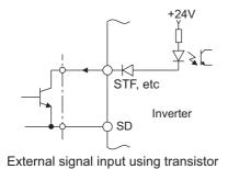
External signal input using transistor
