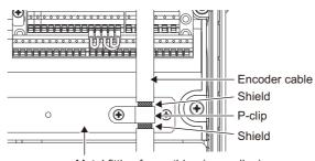
Metal fitting for earthing (grounding)
