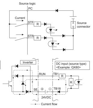
· When using an external power supply for transistor output
