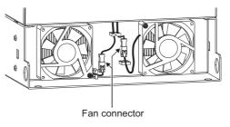
(3) Attach the fan cover with the installation screws. (tightening torque 1.4 to 1.9 N•m)
