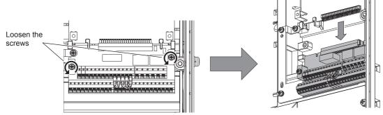
(2) Be careful not to bend the pins of the inverter's control circuit connector, reinstall the control circuit terminal block and fix it with the installation screws.
