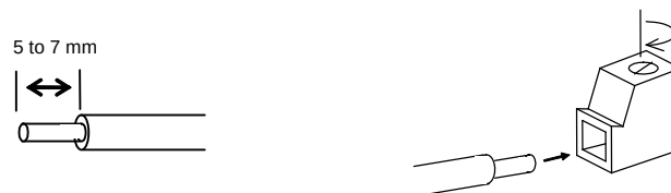
Figure 1.6 Stripping the Wire End Before Connection to Terminal Board
