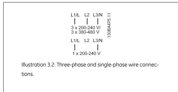
Illustration 3.2: Three-phase and single-phase wire connections.
