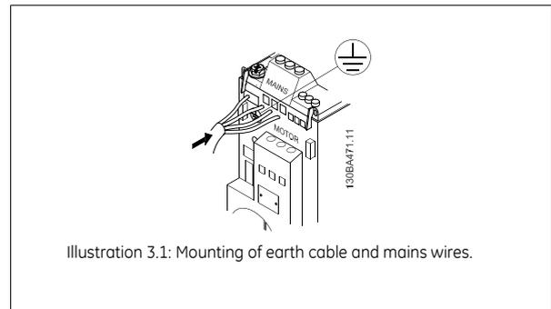
Illustration 3.1: Mounting of earth cable and mains wires.
