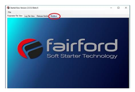
The cable allows the real time interaction between StarterView and either synergy $^{\text{TM}}$  or agility $^{\text{TM}}$  units. Note that the cable(s) must be plugged into the PC before StarterView is run. Subsequent cables/devices can then be added once the Modbus tab becomes active.
