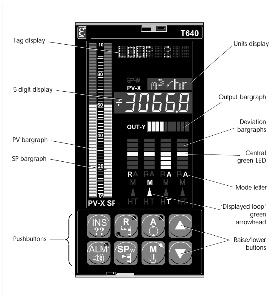
Figure 4-1 T640 front panel — the operator interface
