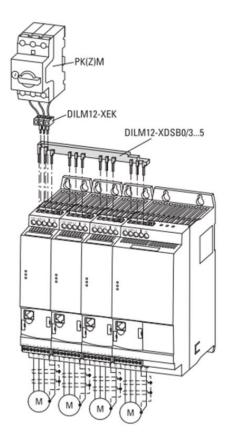
In all situations described above a direct side by side mounting of the Variable Speed Starters is permitted. This enables the use of commoning links DILM12-XDSB0/3...5 for parallel supply of multiple VSS and the use of a common protective device up to a max. current of 30 A.
