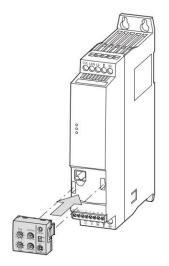
DXE-EXT-SET is an optional module, which can be plugged onto the front of the Variable Speed Starter. It is used for simple modification of selected parameters without using a PC or keypad. All sizes of DE11 use the same module.
