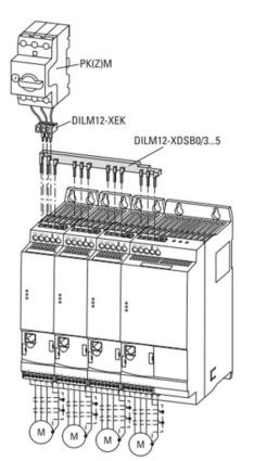
In all situations described above a direct side by side mounting of the Variable Speed Starters is permitted. This enables the use of commoning links DILM12-XDSB0/3...5 for parallel supply of multiple VSS and the use of a common protective device up to a max. current of 30 A.
