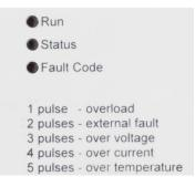
The LEDs on the front of the Variable Speed Starter indicate operating status and faults
