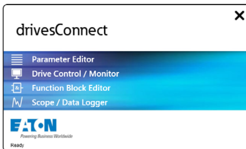
Figure 60: Main drivesConnect components on start screen
