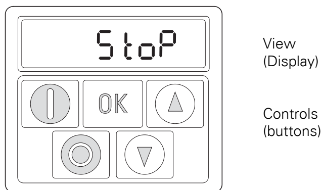
Figure 57: DX-KEY-LED operating unit view
