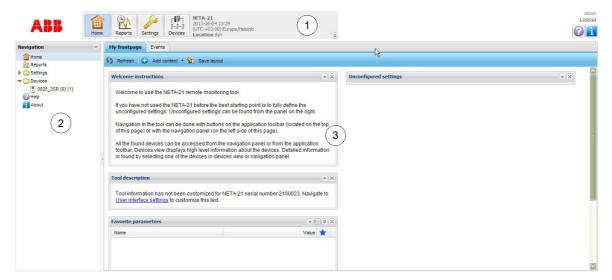
The front page is a portal where you can change the contents by adding, removing or moving around the portlets. The figure below shows a modified front page.
