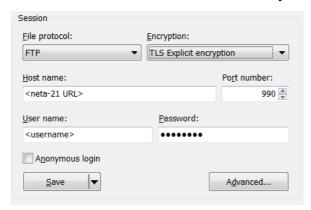
When you configure the FTP connection, you have to specify the protocol, the URL (or IP address) of the NETA-21 and the username and password of the FTP account.
