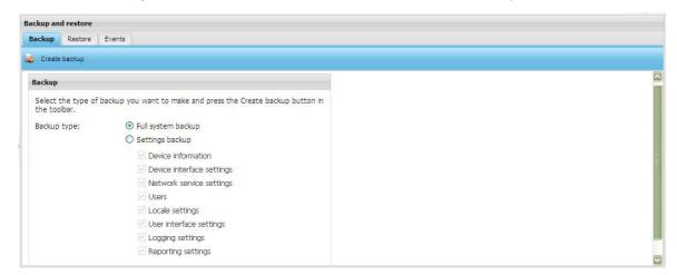
Note: You must have an SD/SDHC card installed into the SD slot to create a backup. The SD card must have a minimum of 200 MB free space to enable the backup/restore functions. Backup and restore files are stored in the BACKUP folder on the SD card.
