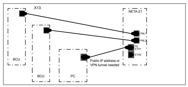
In the BCU-02/12/22 control unit, use connector X13 for the panel bus connection.
