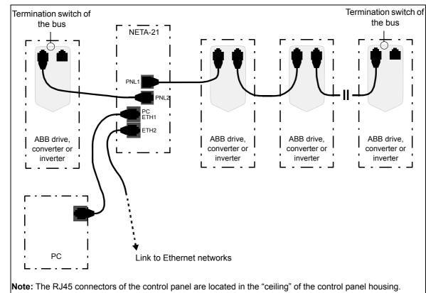
**Note:** The RJ45 connectors of the control panel are located in the "ceiling" of the control panel housing. Beside the left-hand side RJ45 connector in the control panel housing there is a switch that must be pushed upwards in the last drive of the chain to terminate the bus.
