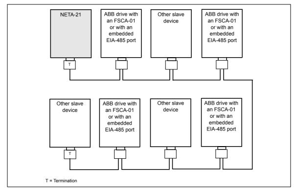
The X3 EIA-485 connector for a Modbus network is located at the bottom of the NETA-21. See the bottom layout in section *Layout of the NETA-21 and the NEXA-21*. The EIA-485 (RS-485) cabling requires a shielded dual twisted pair cable. The nominal impedance of the cable must between 100...150 ohm.
