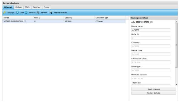
**Note:** If there is an ACS880 drive equipped with a FENA-11/21 adapter module in the Ethernet network, the NETA-21 and the Drive composer PC tool cannot access the FENA-11/21 at the same time. The FENA-11/21 can have only one PC tool connection at a time. The FENA-11/21 connection can be released for a PC tool by removing the specific Ethernet device from the NETA-21 device interfaces view (or by clicking the **Remove** button on a specific Ethernet device front page).
