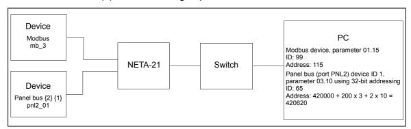
By default, the Modbus protocol returns the internal raw 16-bit value and does not specify any information about sign and scaling. Therefore, you must apply the correct ones for the specified parameter.
