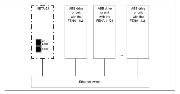
The NETA-21 detects nearby adapter modules (max. 32 pcs over Ethernet) in a local network. The automatic detection is enabled by default only via the ETH2 port. To change the settings of the automatic detection, go to **Settings –> Device interfaces –> Ethernet** –> **Settings –> Background scan**.
