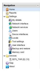
**Note:** If the NETA-21 does not detect all drives automatically, go to **Settings -> Device interfaces -> ddcs -> Rescan devices**.
