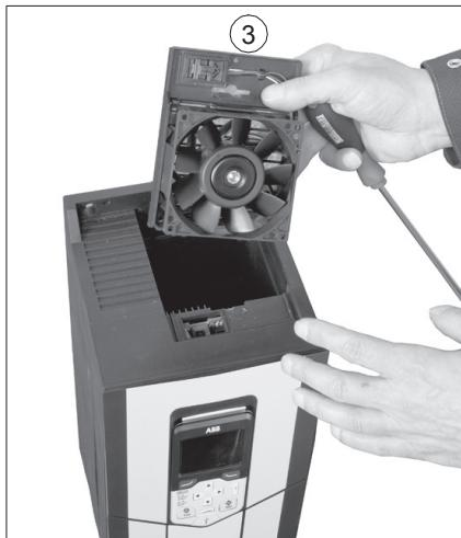
**■ Replacing the auxiliary cooling fan of IP55 frames R1 to R3**
