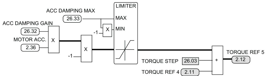
In the block diagram above, the Acceleration damping function is extracted from the complete speed and torque control chain. For a more detailed control chart, see the *ACS800 System Control Program 7.x Firmware Manual* (3AFE64670646 [English]). See also section *Calculation of the motor shaft actual acceleration* on page 13.
