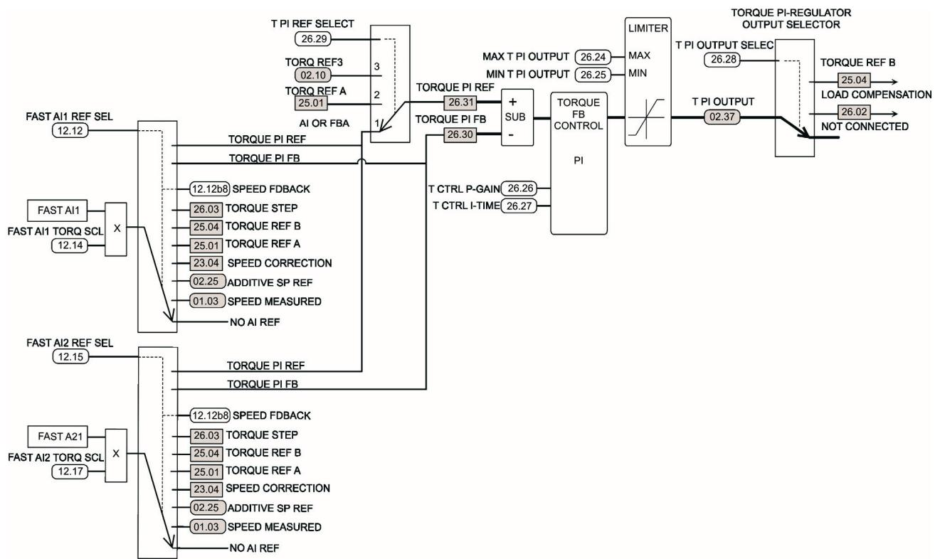
Fast PI regulator for torque correction (running at 1 ms time level). Extracted from the complete speed and torque control chain. For the complete control chart, see *ACS800 System Control Program 7.x Firmware manual* (3AFE64670646 [English]).
