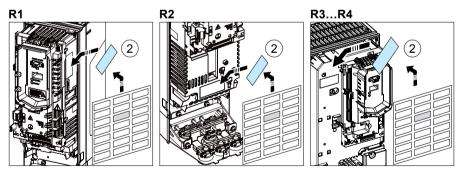
3. Remove the rubber grommets from the cable entry if they point up. (The grommets may point up or down when you open the package, depending on the frame size.)
