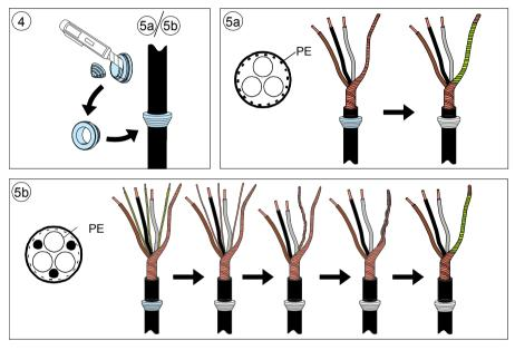
6. Slide the cable through the hole in the cable entry and attach the grommet to the hole.
