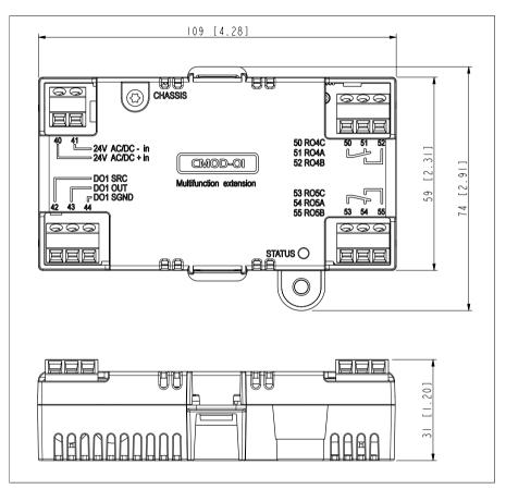
Installation: Into an option slot on the drive control board
