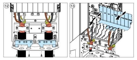
15. Ground the motor cable shield at the motor end. For minimum radio frequency interference, ground the motor cable shield 360 degrees at the cable entry of the motor terminal box.
