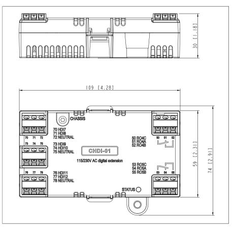
Installation: Into an option slot on the drive control board
