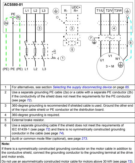
Do not use an asymmetrically constructed motor cable for motors above 30 kW (see page 72). Connecting its fourth conductor at the motor end increases bearing currents and causes extra wear.
