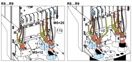
12. Install the grounding shelf of the control cables.
