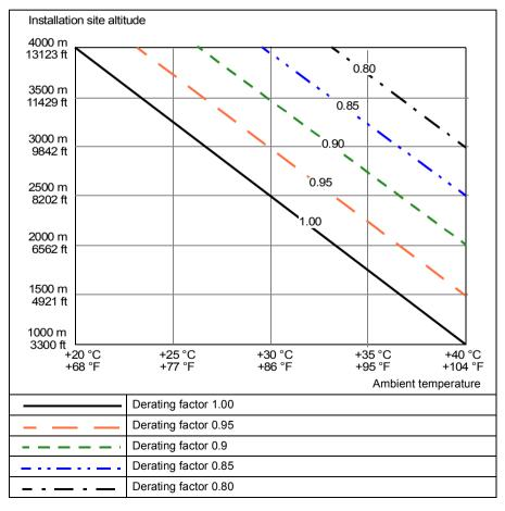
The altitude derating can be reduced if the temperature is below +40 °C, for example, if the temperature is 30 °C, the derating factor is  $1 - 1.5\% \cdot 10 = 0.85$ . You can reduce the output current by 35% instead of 40% at 4000 meter above the see level.
