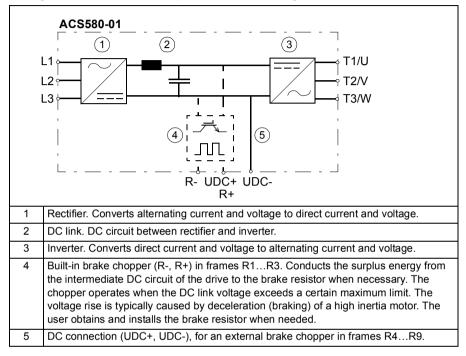
The figure below shows the simplified main circuit diagram of the drive.
