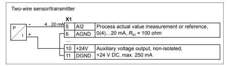
**Note:** The sensor is supplied through its current output and the drive feeds the supply voltage (+24 V DC). Thus the output signal must be 4...20 mA, not 0...20 mA.
