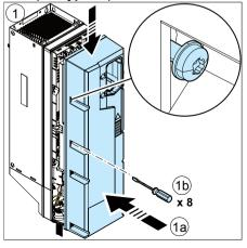
Reinstalling side plates and covers, frames R6...R9
