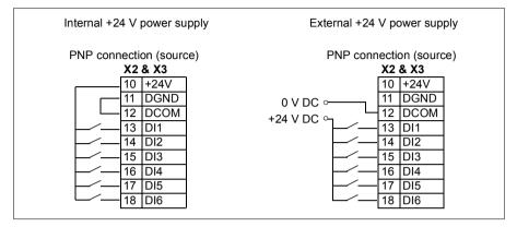
**WARNING!** Do not connect the +24 V AC cable to the control board ground when the control board is powered using an external 24 V AC supply.
