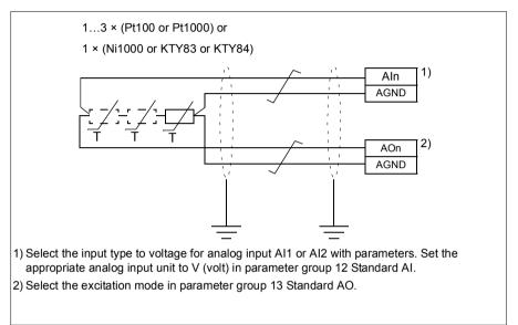
WARNING! As the inputs pictured above are not insulated according to IEC 60664, the connection of the motor temperature sensor requires double or reinforced insulation between motor live parts and the sensor. If the assembly does not fulfill the requirement, the I/O board terminals must be protected against contact and must not be connected to other equipment or the temperature sensor must be isolated from the I/O terminals.
