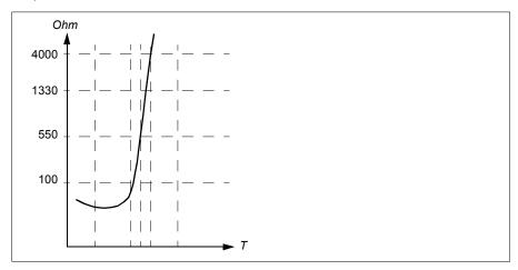
One isolated PTC sensor can also be connected directly to digital input DI6. At the motor end, the cable shield should be earthed through a capacitor. If this is not possible, leave the shield unconnected.
