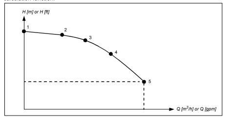
The figure below shows the PQ performance curve of the pump for the flow calculation function.
