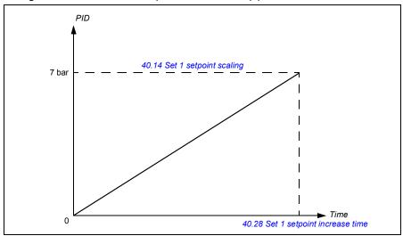
If the pumping system is leaking or is damaged then the setpoint will not reach in time. To detect such a condition, you can enable soft pipe fill supervision to generate a warning or a fault. The time is calculated with the last reference change in parameter 40.03 Process PID setpoint actual.
