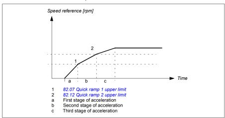
In submersible (a.k.a borehole) pumps, the mechanical wearing of bearings can be reduced by ramping the pump guickly to a certain speed.
