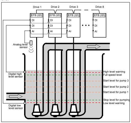
The first pump (master) will start when the actual level is above the start point 1. More pumps will start and stop based on the rising (emptying) or falling (filling) water levels of individual pumps. In case of a pump failure or if drive is disconnected for maintenance, the system still continues operation with the remaining pumps and drives.
