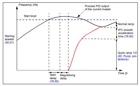
The timing diagram of Smooth pump transitions shows the pump starting steps. In this case, the process PID output of the current master has exceeded the start level (76.30...76.36).
