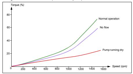
The dry run can be detected using the underload curve, low level mechanical switch and pressure sensor.
