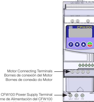
Figure A4: Indication of the connecting terminals of the CFW100
