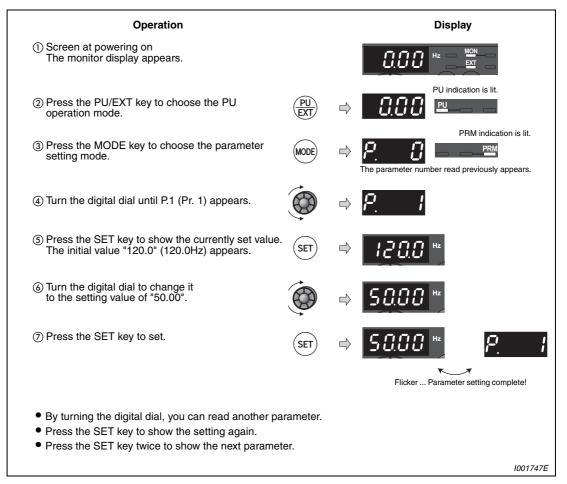
Fig. 5-6: Setting the maximum frequency
