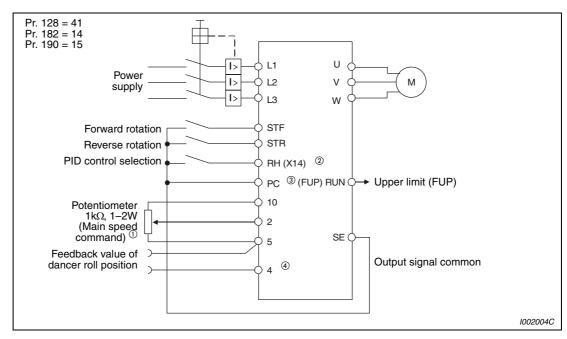
Fig. 6-133: Example in source logic
