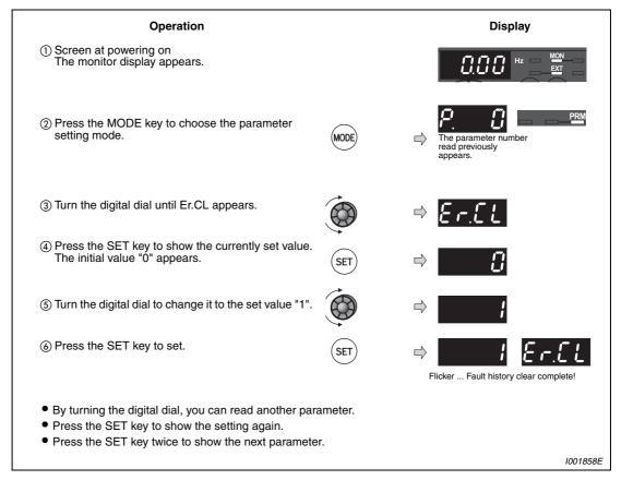
Fig. 7-6: Clearing the fault history
