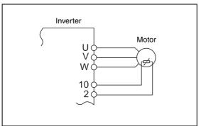
Fig. 6-37: PTC thermistor input connection
