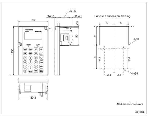
Fig. A-5: Parameter unit FR-PU07
