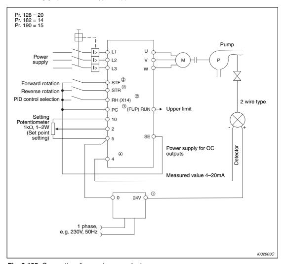
Fig. 6-125: Connection diagram in source logic
