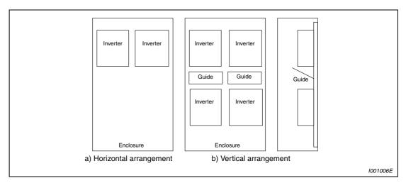
Fig. 2-10: Arrangement of multiple inverters
