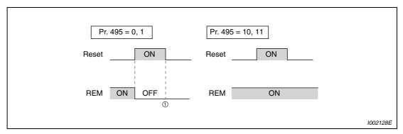
Fig. 6-59: Signal condition during a reset
