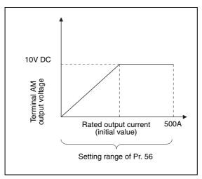
Fig. 6-64: Current monitoring reference
