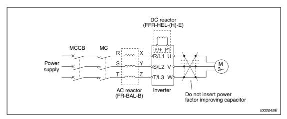
Fig. 3-41: Reduction of power supply harmonics
