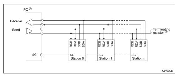
Fig. 6-102: Connection to several inverter
