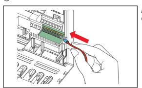
Fig. 3-10: Cable connection
