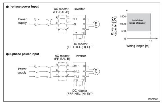
Fig. 3-35: Installation of a reactor
