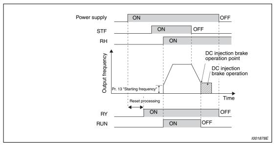
Fig. 4-3: Ready status and motor running
