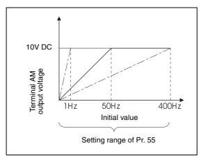
Fig. 6-63: Frequency monitoring reference
