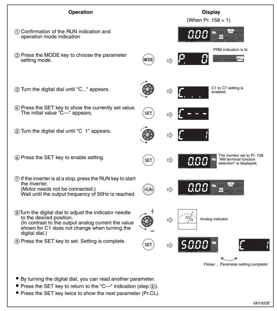
Fig. 6-67: AM terminal calibration
