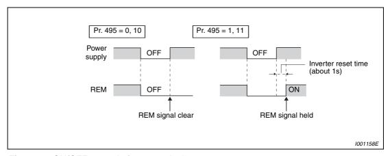
Fig. 6-58: ON/OFF example for source logic
