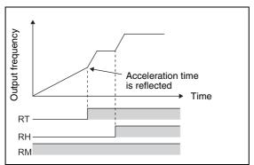
**Fig. 6-46:**Second acceleration/deceleration time example
