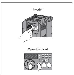
Fig. 6-93: PU operation mode
