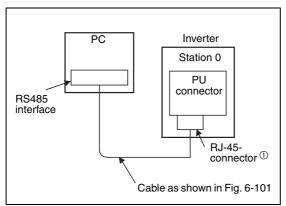
Fig. 6-98: Connecting the RS485 interface of a PC to the PU connector
