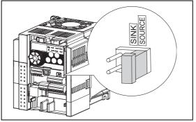
Fig. 3-18: Changing the control logic
