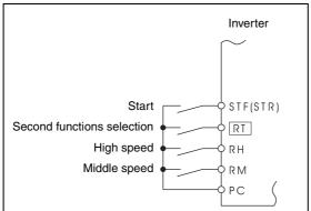
Fig. 6-45: Second functions connection diagram
