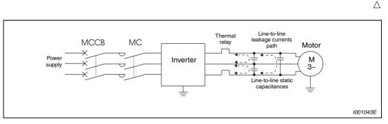
Fig. 3-36: Line-to-line leakage currents
