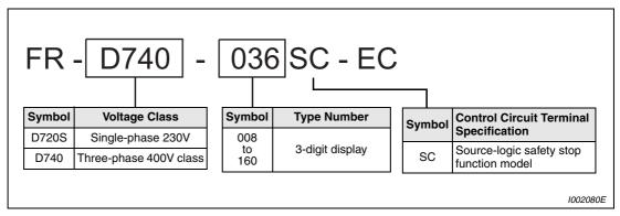
Fig. 1-1: Inverter type FR-D700 SC EC
