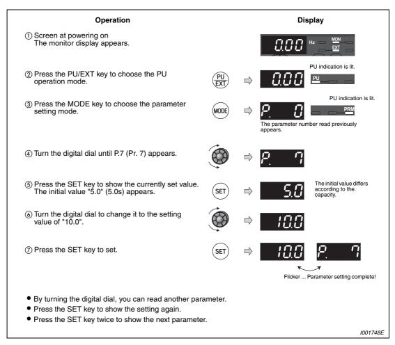
Fig. 5-8: Setting the acceleration time
