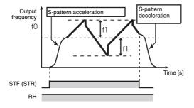
When stall prevention is activated during traverse operation, traverse operation is stopped and normal operation is performed. When stall prevention operation ends, the motor accelerates/decelerates to f0 in normal acceleration/deceleration time (Pr. 7, Pr. 8). After the output frequency reaches f0, traverse operation is again performed.
