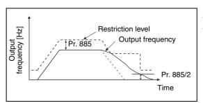
Fig. 6-138: Limit the output frequency
