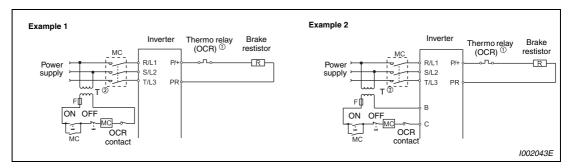
Fig. 3-27: Protection circuits
