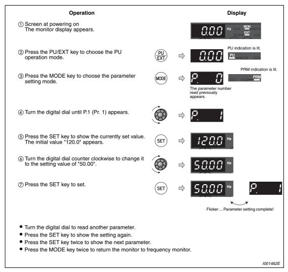
Fig. 4-12: Setting the maximum output frequency
