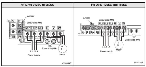
Tab. 3-4: Terminal layout and wiring
