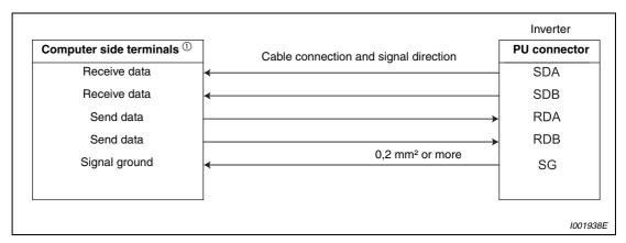
Fig. 6-101: Connection to an inverter
