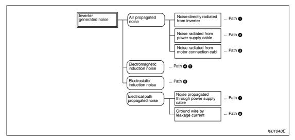
Fig. 3-38: Noise propagation
