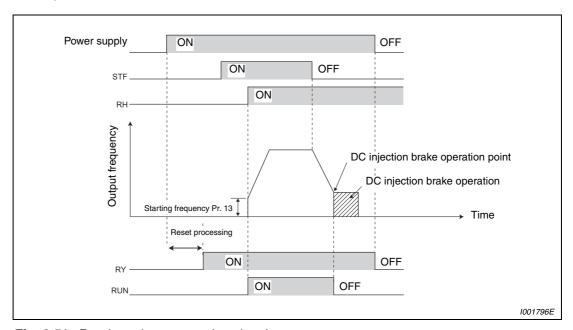
Fig. 6-51: Ready and motor running signals
