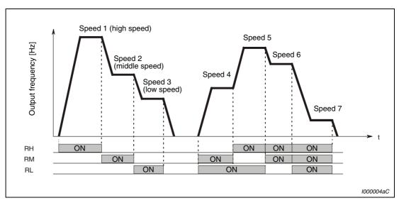
Fig. 5-23: Multi-speed selection by external terminals
