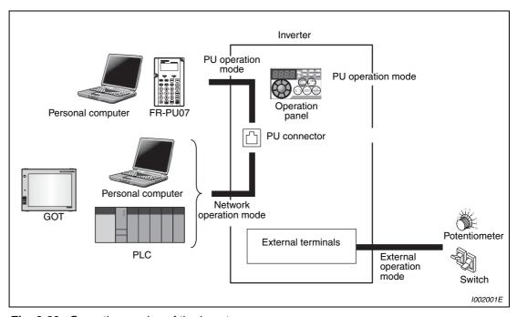
Fig. 6-89: Operation modes of the inverter
