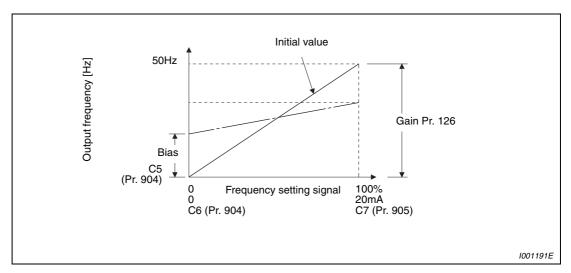
Fig. 6-84: Signal adjustment of terminal 4
