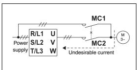
Fig. 4-1: Mechanical interlocks for MC1 and MC2
