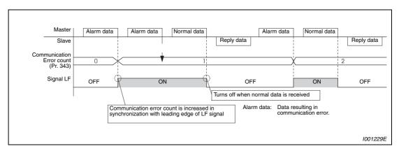
Fig. 6-118: Output of the LF signal
