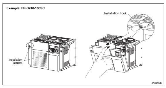
Fig. 2-3: Removal of the front cover
