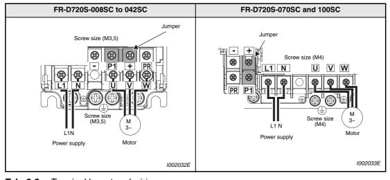
Tab. 3-3: Terminal layout and wiring
