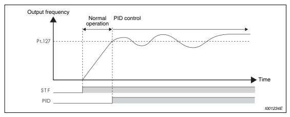
Fig. 6-126: Automatic switchover to PID control
