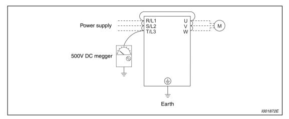
Fig. 8-7: Insulation resistance test
