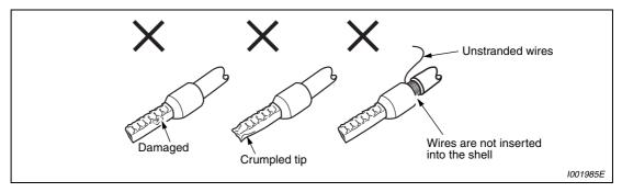
Fig. 3-9: Incorrectly crimped wire end sleeves
