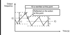
When the output frequency exceeds Pr. 1 Maximum frequency or Pr. 2 Minimum frequency, the output frequency is clamped at maximum/minimum frequency while the set pattern exceeds the maximum/minimum frequency.
