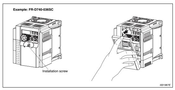
Fig. 2-1: Removal of the front cover
