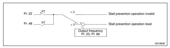
Fig. 6-3: Stall prevention block diagram
