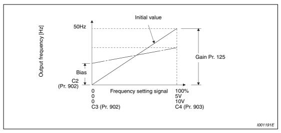
Fig. 6-83: Signal adjustment of terminal 2
