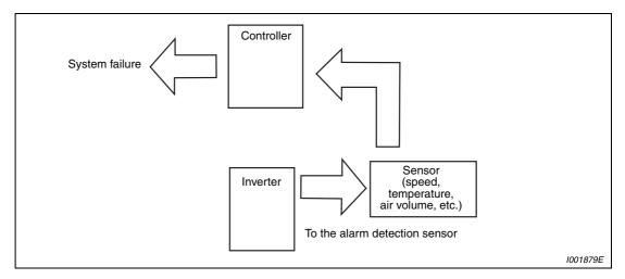
Fig. 4-4: Backup method outside the inverter
