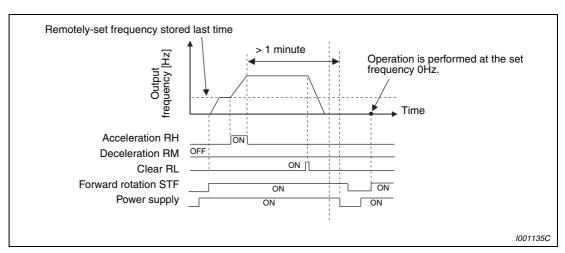
Fig. 6-26: Outputting the current set frequency
