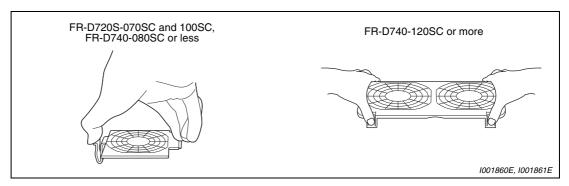
Fig. 8-2: Removal of the fan cover
