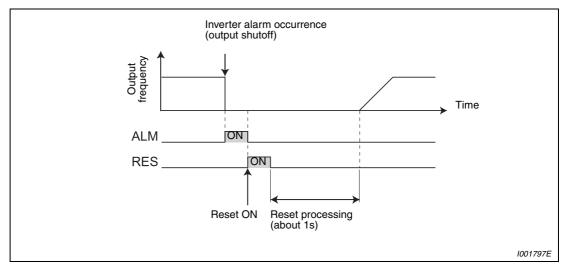
Fig. 6-52: Alarm signals
