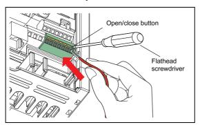
Fig. 3-11: Connection of a stranded wire
