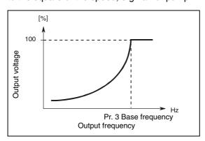
Fig. 6-13: Variable-torque load
