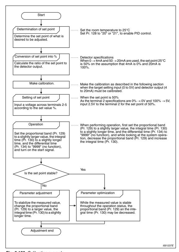
Fig. 6-129: Calibration example
