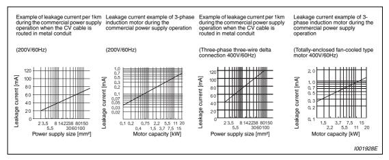
Fig. 3-37: Leakage currents
