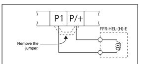
Fig. 3-34: Connection of a DC reactor
