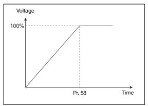
Fig. 6-70: Voltage rise at automatic restart
