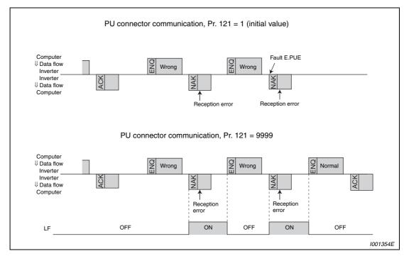
Fig. 6-104: Data transmission error
