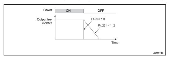
Fig. 6-71: Parameters for stop selection at power failure
