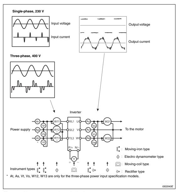
Fig. 7-7: Measurements at the main circuit
