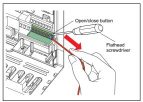
Fig. 3-12: Wire removal
