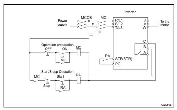
Fig. 3-23: Example for connection of an inverter
