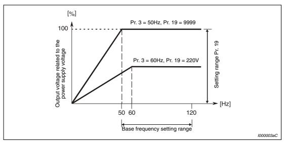
Fig. 6-11: Output voltage related to the output frequency
