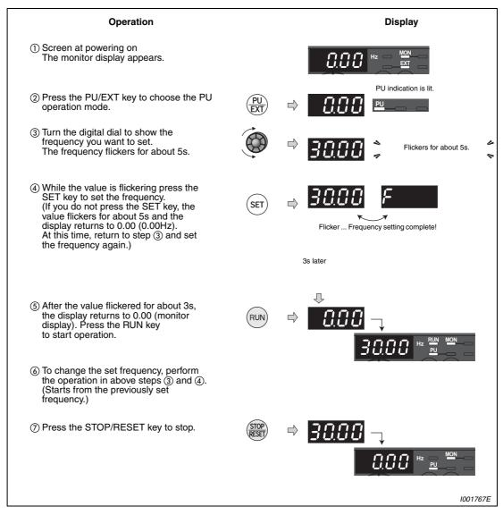
Fig. 5-11: Frequency setting with the digital dial
