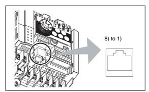
Fig. 6-96: PU connector pin-outs
