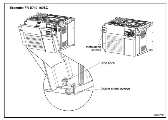
Fig. 2-4: Reinstallation of the front cover
