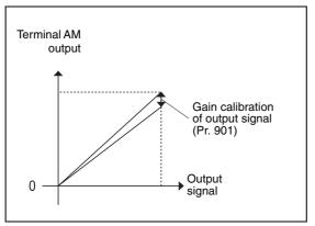
Fig. 6-66: Terminal AM gain calibration
