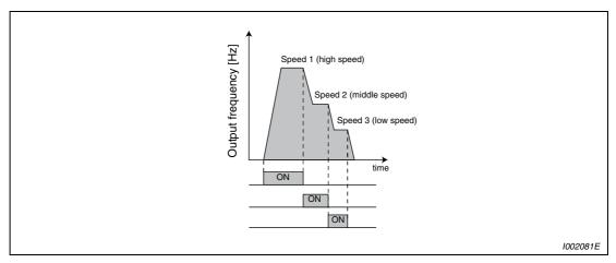
Fig. 6-15: Multi-speed selection by external terminals
