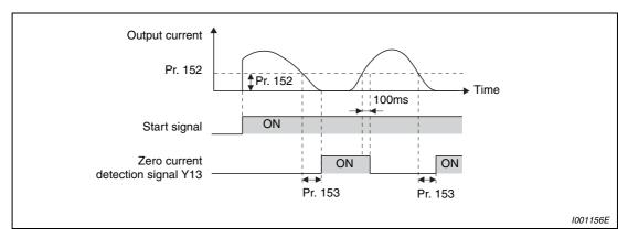
Fig. 6-56: Zero current detection
