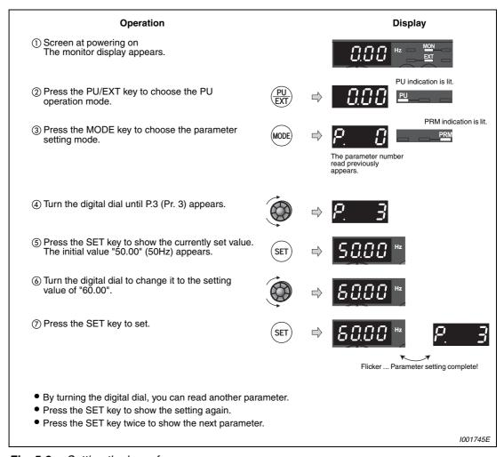
Fig. 5-2: Setting the base frequency
