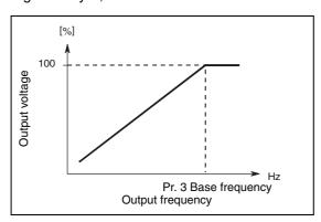
Fig. 6-12: Constant-torque load
