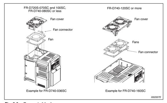
Fig. 8-3: Removal of the fan
