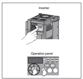
Fig. 5-10: PU operation mode
