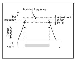
Fig. 6-53: Output of the SU signal
