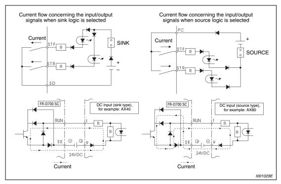
Fig. 3-17: Changing the control logic
