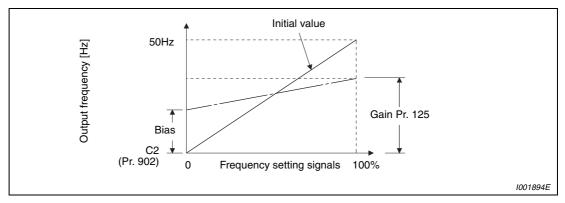
Fig. 6-134: Signal calibration at terminal 2
