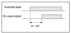
Fig. 6-5: Output of the OL signal
