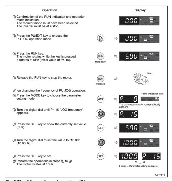
Fig. 6-22: JOG operation performed from PU
