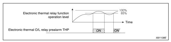
Fig. 6-35: Prealarm signal output
