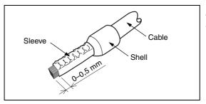
Fig. 3-8: Fixing of wire end sleeves
