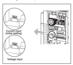
Fig. 6-79: Voltage/current input switch
