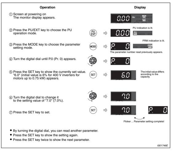
Fig. 5-4: Setting the starting torque
