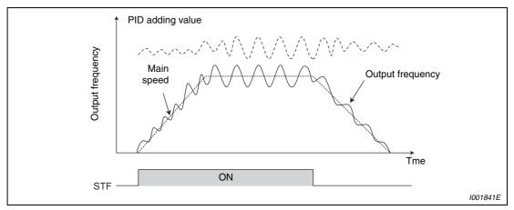
Fig. 6-132: Signal overlay during dancer control
