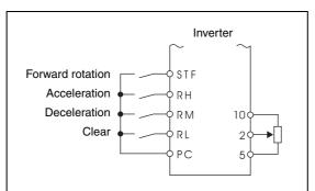
Fig. 6-23: Connection diagram for remote setting
