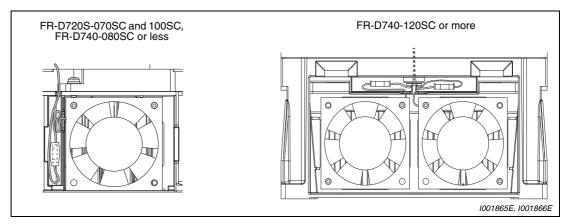
Fig. 8-5: Connection of the fan
