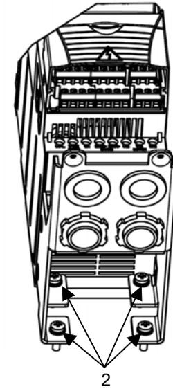
2. Fasten the gland box frame to wall with four M4 screws (not included).
