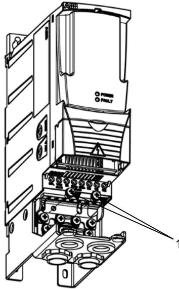
1. Fasten the gland box frame to drive with two M4×12 screws.
