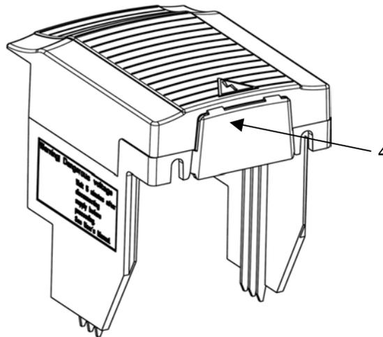
4. With FPBA-01 or FCAN-01 option modules, remove the detachable lid (4) from the gland box cover.
