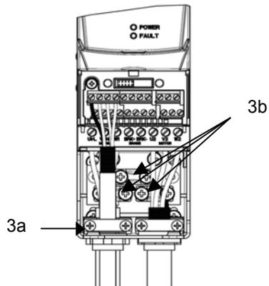
3. Install clamps (3a) for control cables (see power cable lead-throughs), or if cables are run in conduits, replace all clamps with suitable glands (not included). Run cables through the clamps and tighten. Strip cable ends. Fasten the grounding conductor (PE) of the input power cable and the twisted shield of motor cable under the grounding clamps (3b). Connect the conductors to appropriate terminals. See *Electrical installation* in the drive manual.
