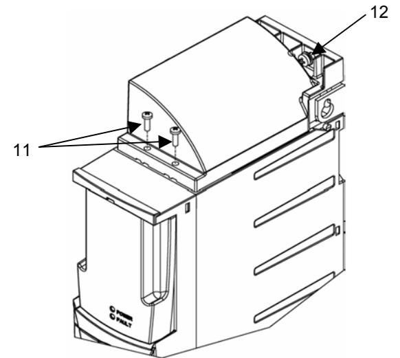
11. Fasten the hood to drive with two M3×12 screws.
