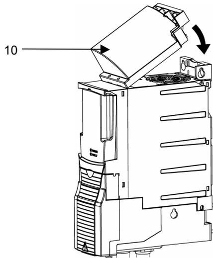
10. Install the hood. First position the front edge carefully, then press the hood downwards until it snaps on.
