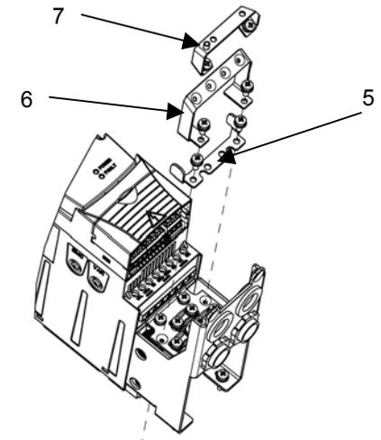
5, 6, 7. With any fieldbus option module except FRSA-00, remove the support plate (5), install the I/O clamping plate (6) and the option grounding plate (7) to the gland box frame. See *Mechanical installation* in the drive manual.
